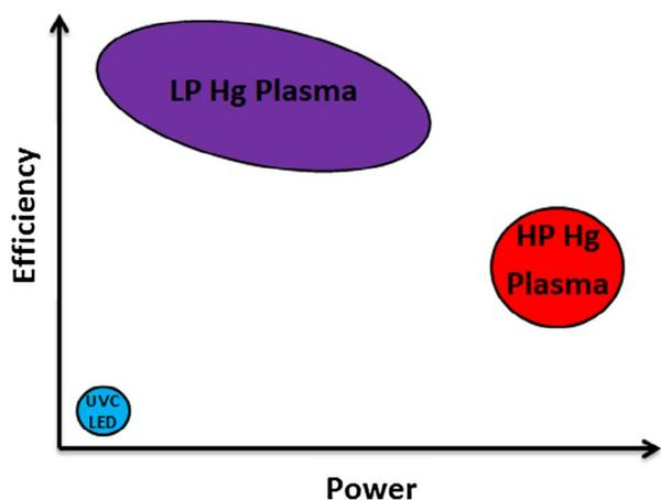
Fig. 1. A conceptual representation of the current status of UVC sources.
