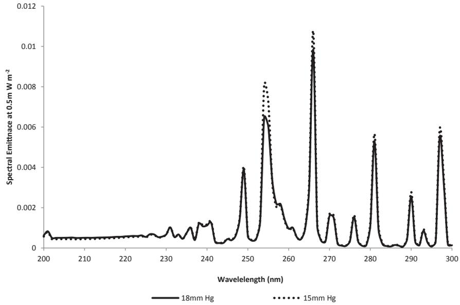
Fig. 7. Mean spectral output of mercury lamps.
