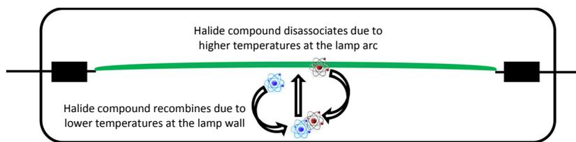
Fig. 2. Diagrammatic representation of halide cycle from lamp wall to lamp arc.
