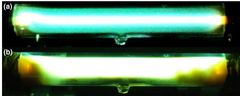
**Fig. 10.** Lamp 15mm IIB. (Image A (Top) taken during the warm up stages of the lamp and Image B (Bottom) taken when the lamp had warmed up).
