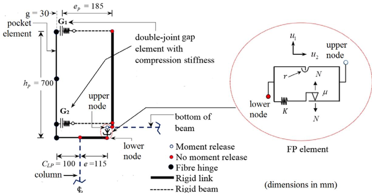
Figure 3. FE mesh of the proposed detailed model of a RC beam-column pocket connection.
