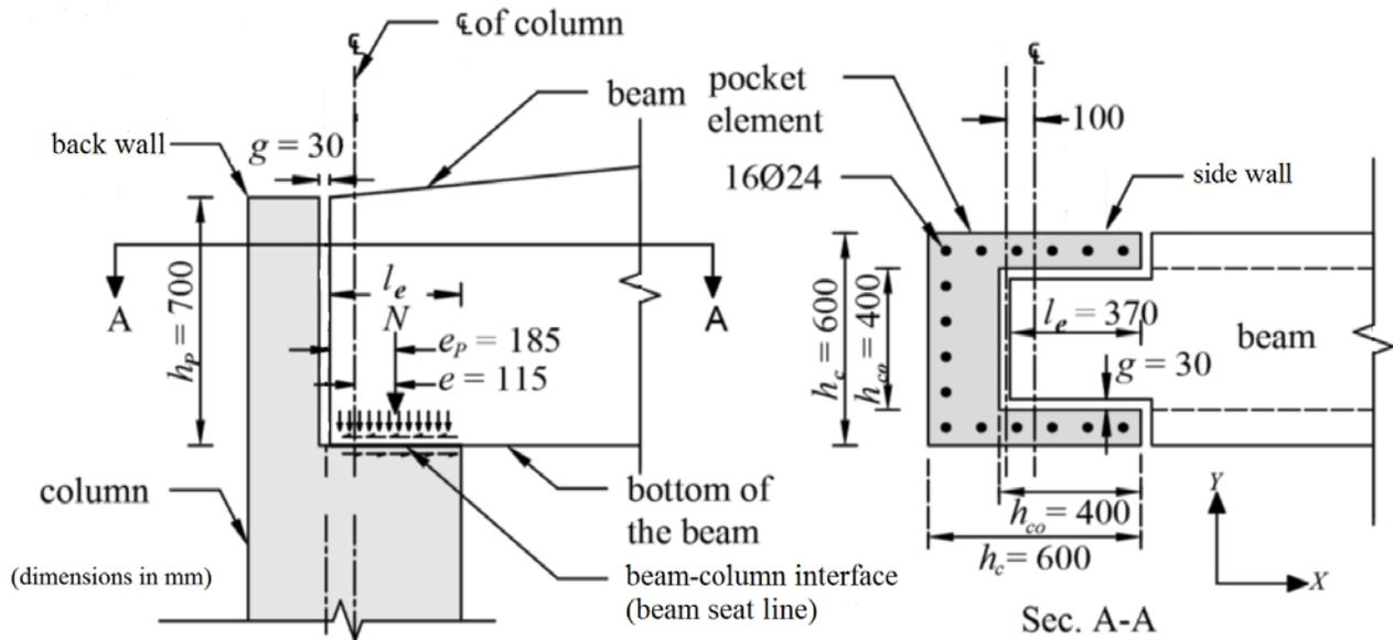
Figure 2. Geometrical details of a beam-column pocket connection.
