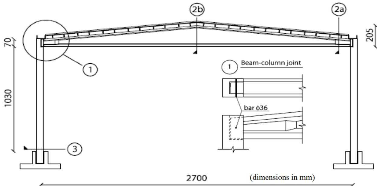
Figure 1. Portal frame made of precast RC members
