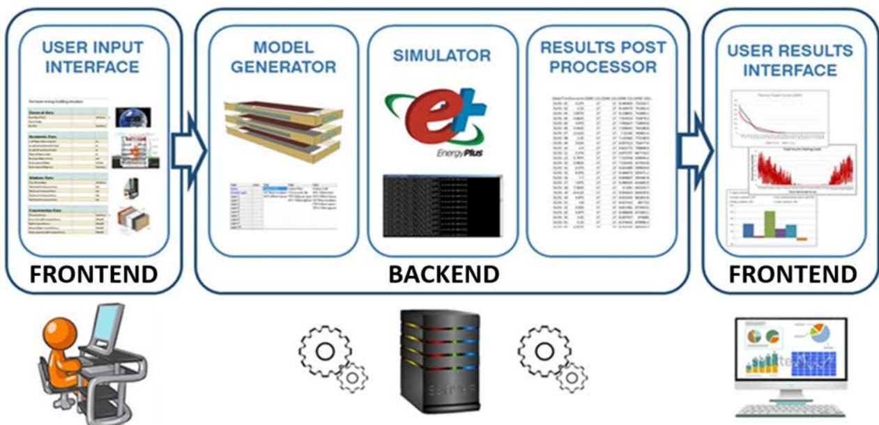
Figure 1: Workflow of the tool and its subsystems
