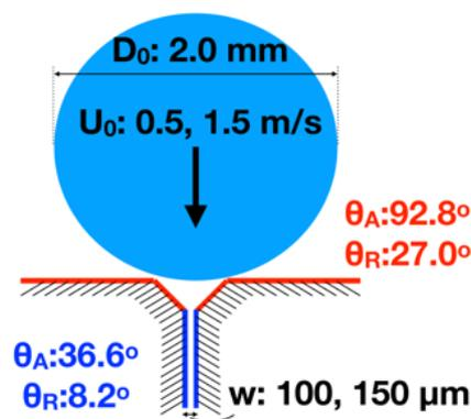
**Figure 1.** Schematic representation and initial conditions of investigated phenomenon
