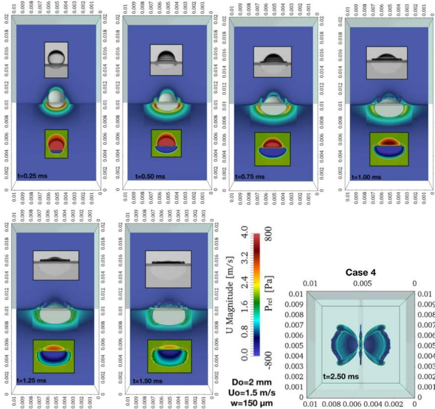
**Figure 6.** Droplet evolution with time for Case 4 (Table 1). Each time instance up to  $t = 1.50$  ms illustrates the experimental snapshots from [12] (top), the numerically predicted droplet interface with a central section of the predicted velocity distribution (middle/main image) and a central section pressure distribution (bottom). For time  $t=2.50$  ms the top view of the droplet surface is depicted, coloured by the velocity magnitude.
