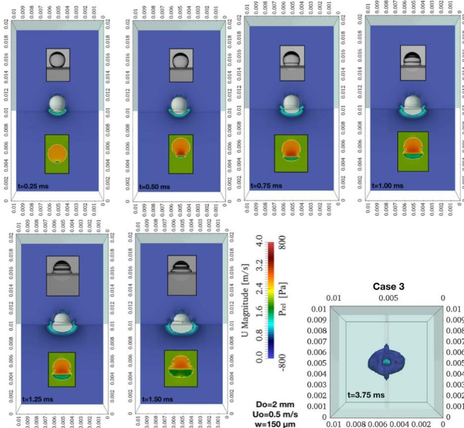
**Figure 5.** Droplet evolution with time for Case 3 (Table 1). Each time instance up to  $t = 1.50$  ms illustrates the experimental snapshots from [12] (top), the numerically predicted droplet interface with a central section of the predicted velocity distribution (middle/main image) and a central section pressure distribution (bottom). For time  $t=3.75$  ms the top view of the droplet surface is depicted, coloured by the velocity magnitude.
