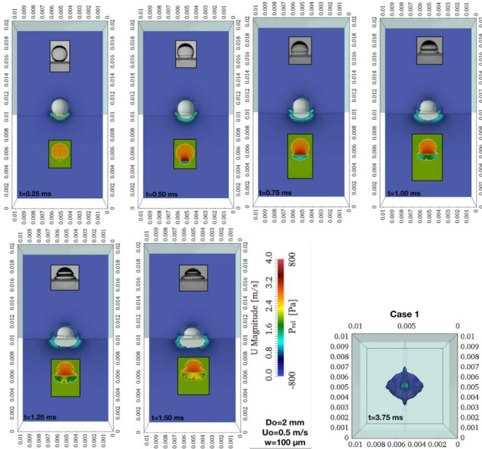
Figure 3. Droplet evolution with time for Case 1 (Table 1). Each time instance up to  $t = 1.50$  ms illustrates the experimental snapshots from [12] (top), the numerically predicted droplet interface with a central section of the predicted velocity distribution (middle/main image) and a central section pressure distribution (bottom). For time  $t=3.75$  ms the top view of the droplet surface is depicted, coloured by the velocity magnitude.
