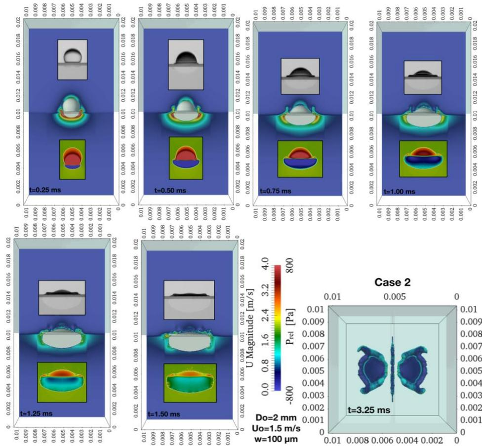
**Figure 4.** Droplet evolution with time for Case 2 (Table 1). Each time instance up to  $t = 1.50$  ms illustrates the experimental snapshots from [12] (top), the numerically predicted droplet interface with a central section of the predicted velocity distribution (middle/main image) and a central section pressure distribution (bottom). For time  $t=3.25$  ms the top view of the droplet surface is depicted, coloured by the velocity magnitude.
