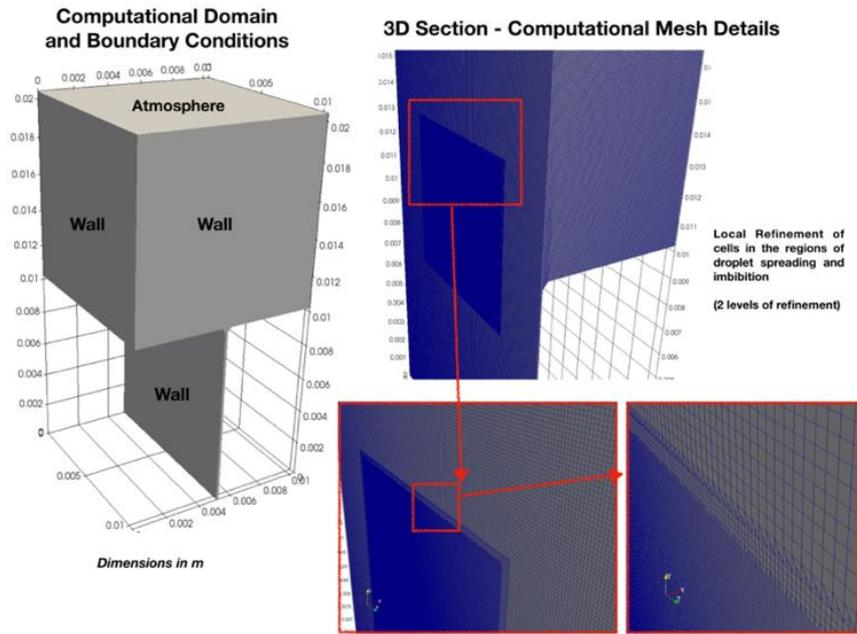
Figure 2. Computational geometry, mesh and boundary conditions.
