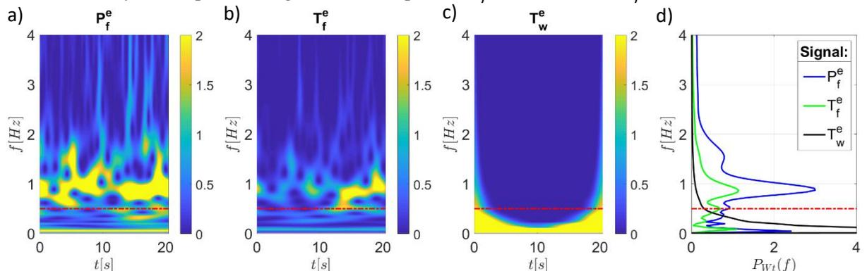
**Figure 3:** a) Wavelet Scalogram of the fluid pressure ( $P_f^e$ ); b) Wavelet Scalogram of the fluid temperature ( $T_f^e$ ); c) Wavelet Scalogram of the wall temperature ( $T_w^e$ ); d) Power Spectrum of the fluid pressure ( $P_f^e$ ) (blue line), the fluid temperature ( $T_f^e$ ) (green line) and the wall temperature ( $T_w^e$ ) (black line).
