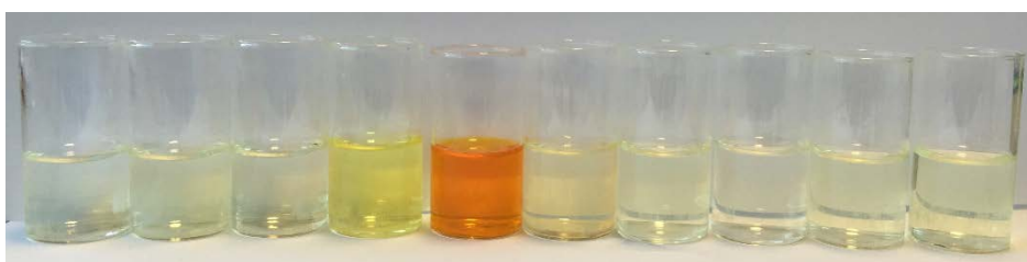
Figure 3: Response of 1c to anions in acetonitrile at 20 °C: (from left) I - , Cl - , Br - , F - , OH - , CH 3 CO 2 - , HSO 3 - , BF 4 - , NO 3 - , PO 4 3-
