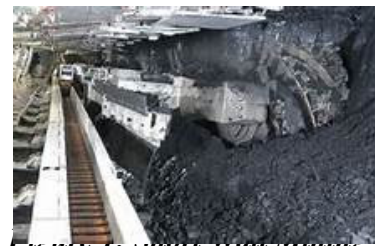
Figure 1. Short wall mining
