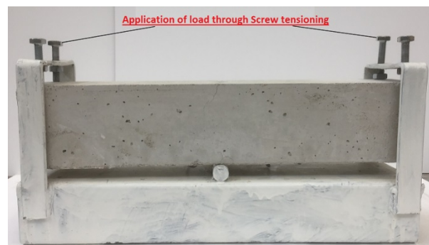
Fig. 1. Method for cracking in the prism samples
