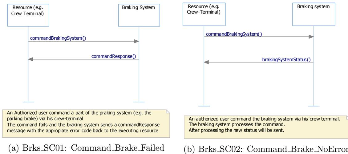
Figure 5.3: NGVA Brakes PIM Sequence Diagrams
