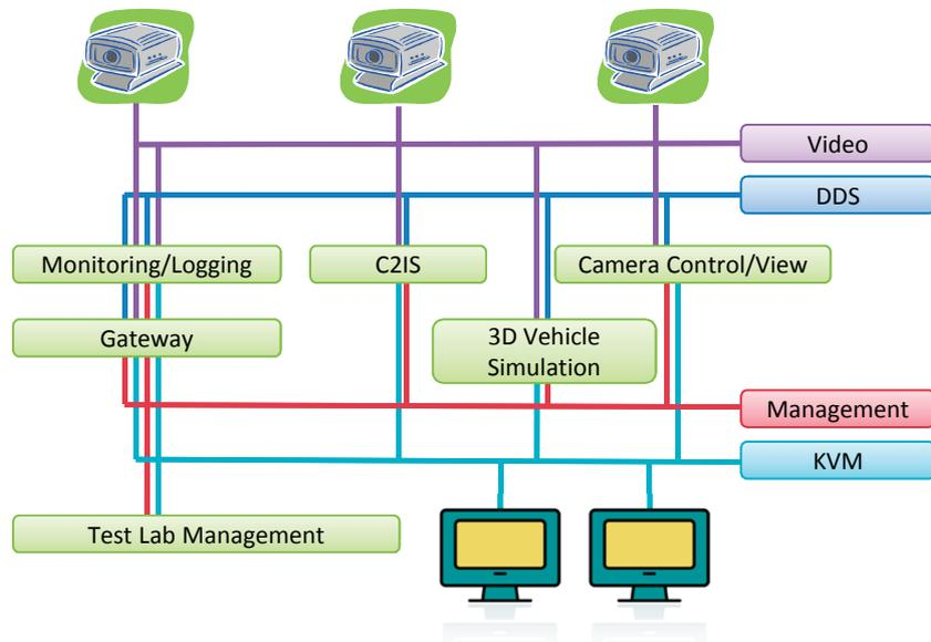
Figure 4.15: Simplified NGVA Interoperability Test Configuration
