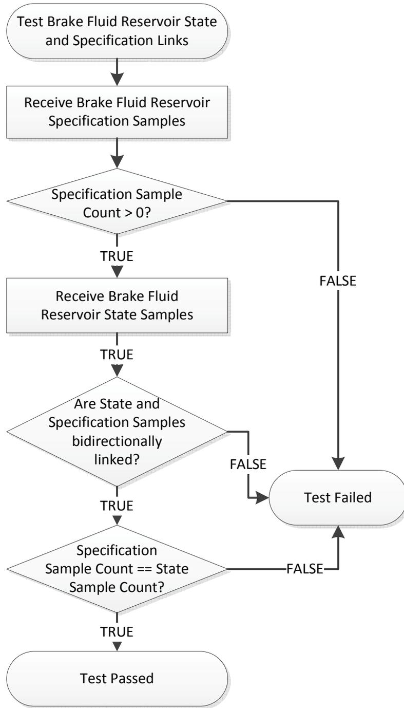
Figure 5.5: Flow Chart of an Example Test Case
