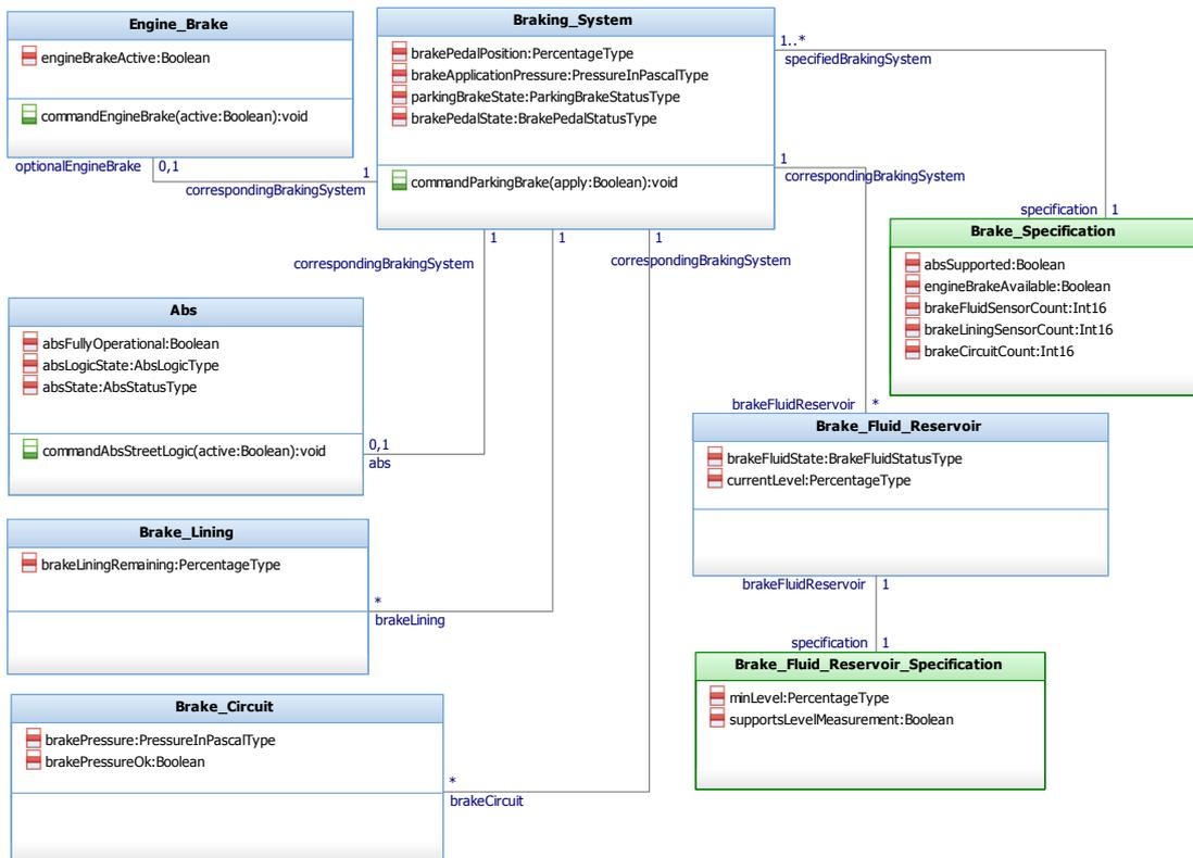
Figure 5.1: NGVA Brakes PIM Class Diagram
