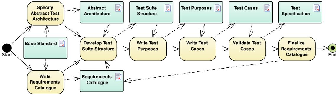
Figure 4.4: Development of a Test Specification (adapted from [22, Section 8])
