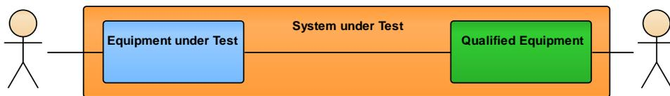
Figure 4.2: Interoperability Testing (adapted from [22, Section 4.1])
