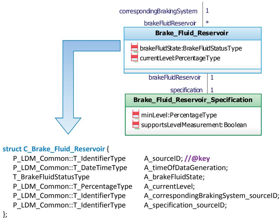
Figure 2.5: Example translation of a PIM class to IDL code
