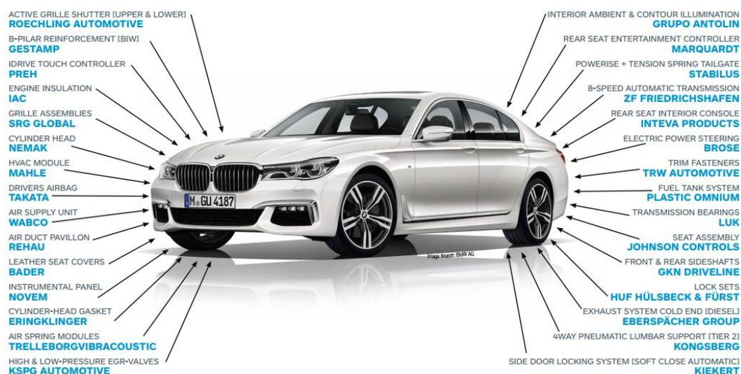
Figure 2-2 A representation of various supplier systems for a luxury vehicle [9]
