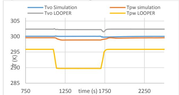
**Fig. 5 -** Primary wick and vapour grooves temperatures comparison
