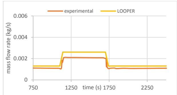
**Fig. 4 -** Mass flow rate comparison
