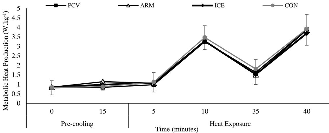
**Figure 6.3** Mean  $\pm$  SD of metabolic heat production before and after the pre-cooling period, and prior to and post the first and last walking period during the heat exposure.
