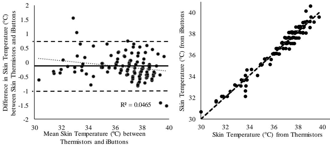
**Figure 3.2** Bland-Altman plot presented with mean bias and LOA (A) and a line of equality graph (B) for mean skin temperature (°C) between thermistors and iButtons.
