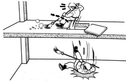
b) Hazard 2 (H2): Fall from uncovered holes
