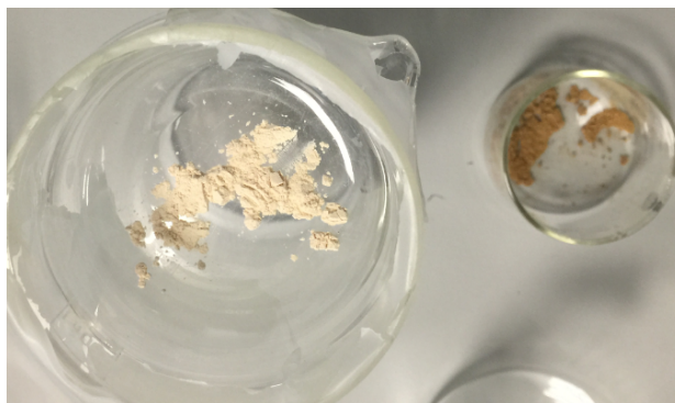
Figure 2-2: The difference between levothyroxine stored at 40°C (Left), and levothyroxine stored at 70°C after t=180 days (Right)
