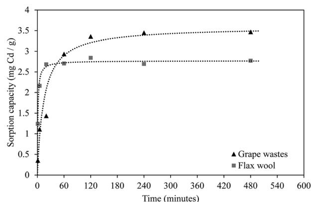
**Fig. 4** Cadmium sorption kinetics onto grape wastes (GW, black triangles) and flax wool (FW, grey squares) as a function of time for an initial concentration of ~18.4 mg L<sup>-1</sup>, pH of 5.5 and temperature of 22 °C ± 2 °C (n = 2). Lines represent pseudo second-order modelled data.
