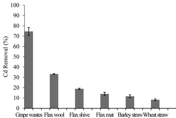
Fig. 2 Removal efficiencies (%) of all tested AWB materials. Initial Cd concentration of  $19.3 \text{ mg L}^{-1}$  in batch conditions (200 mg sorbent: 40 mL of solution, 100 rpm 24 h, pH 2.2). Error bars represent the standard deviation ( $n = 3$ ).
