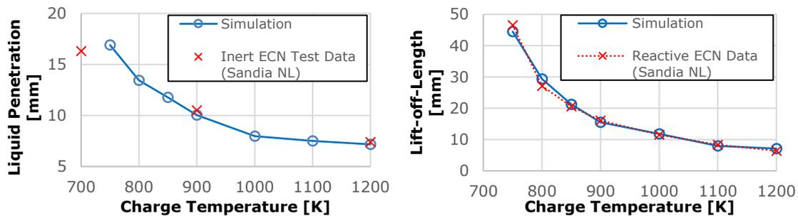
Figure 7: Simulated versus experimental liquid penetration and lift-off-length at all charge temperature conditions
