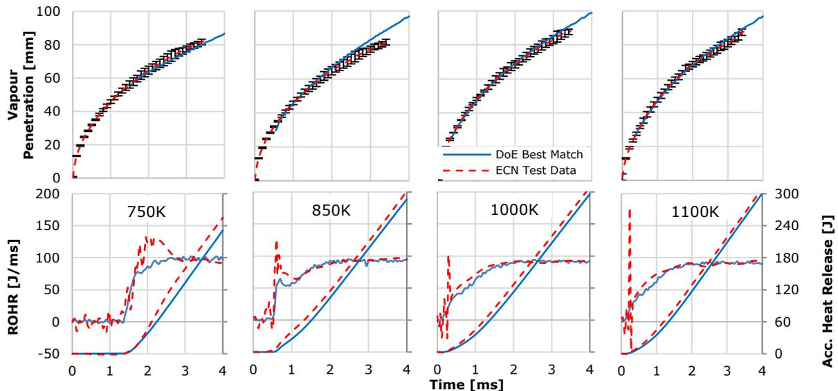
Figure 6: Simulated vs experimental liquid & vapour penetration, ROHR and accumulated HR at the remaining charge temperature conditions
