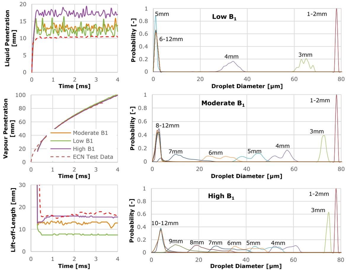
Figure 2: The effect of a discrete swing of KH-time constant  $B_1$  on multiple comparison metrics
