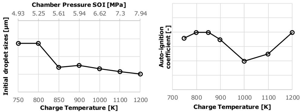
Figure 5: Trend of the required initial droplet sizes and auto ignition coefficient to achieve matching simulations
