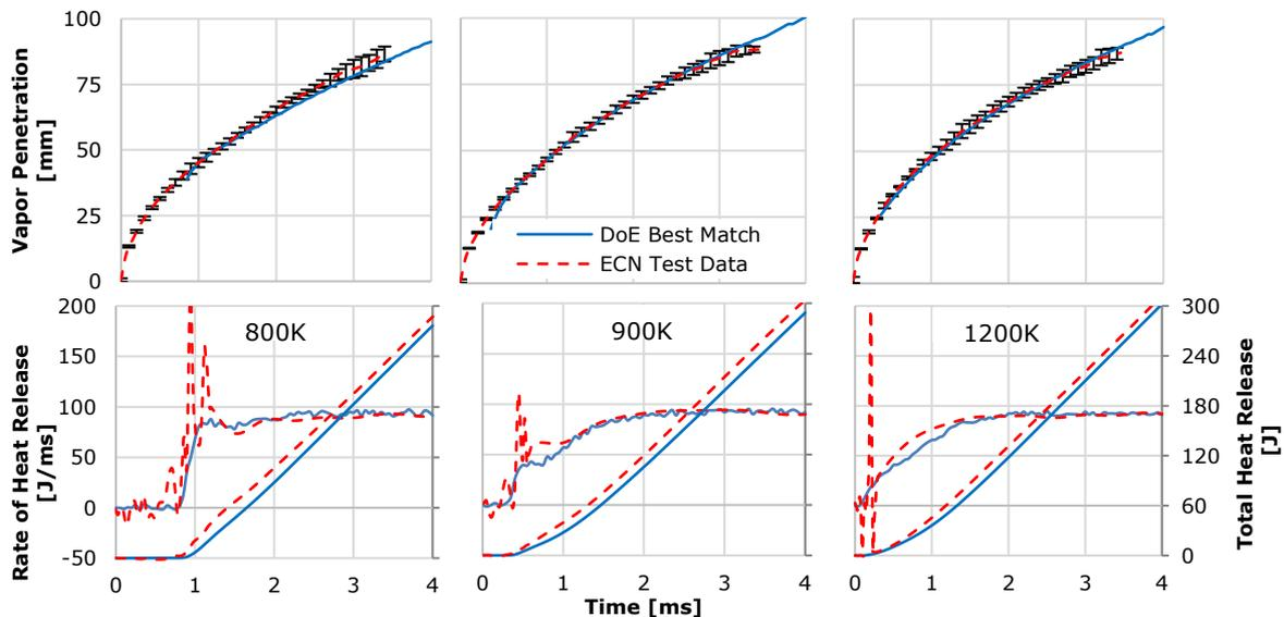
Figure 4: Simulated liquid penetration, vapour penetration, ROHR and AHR against exp. data at 800K (l), 900K (m) and 1200K (r)
