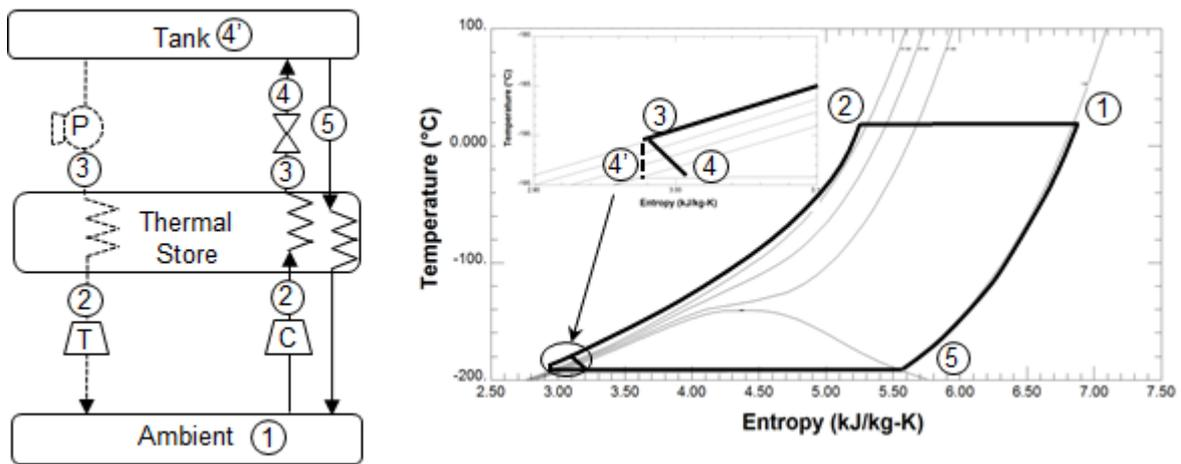
Fig 2. Flow and TS diagram of the LAES cycle
