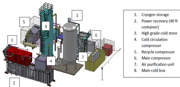
Fig. 7 Pilot plant layout
