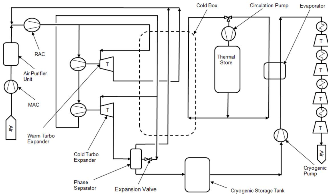
Fig.4. Basic LAES cycle diagram
