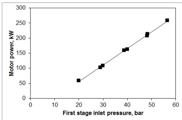
Fig. 8a Effect of stage 1 turbine inlet pressure on generated power at 289K inlet pressure
