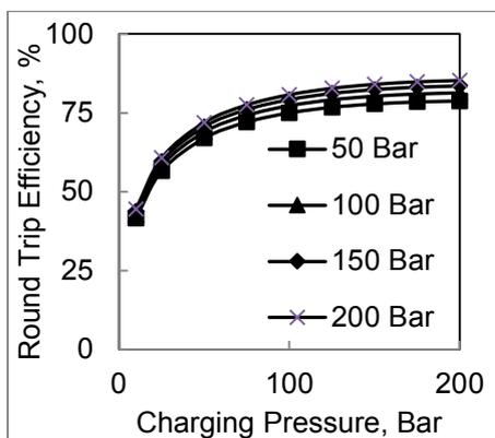
Fig. 3. Theoretical effect of peal charging pressure on round trip efficiency for different liquefier peak pressures
