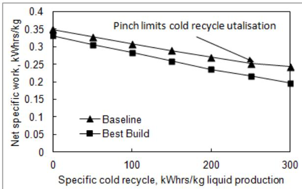
Fig. 10 Effect of specific cold recycle on liquefier efficiency for baseline and 'best' build
