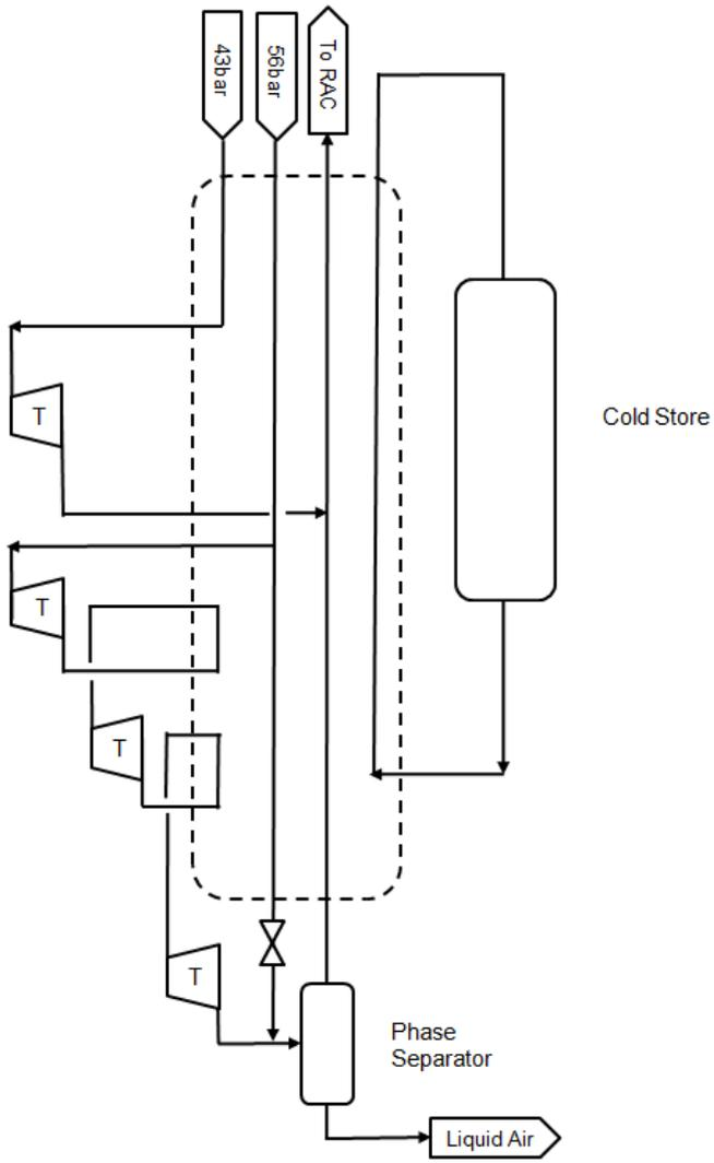
Fig. 11 Best build process layout
