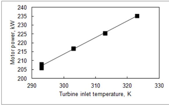
Fig. 8b Effect of turbine inlet temperature on generated power at 48 bar stage 1 inlet pressure
