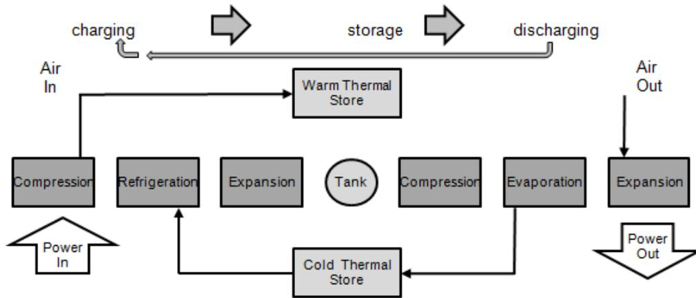
Fig. 1. Block diagram of the LAES system
