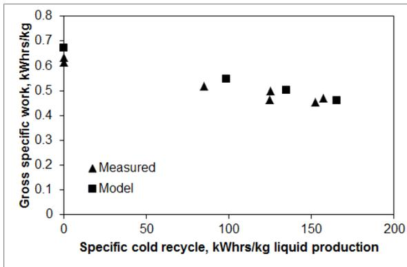
Fig. 9 Measured and predicted gross liquefier specific work
