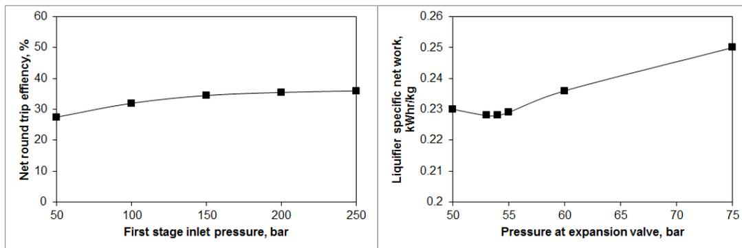
Fig.5. Effect of liquefier and power recovery peak pressures on specific work and round trip efficiency
