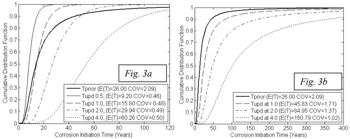
Figure 3: Posterior corrosion initiation time at rebar level
