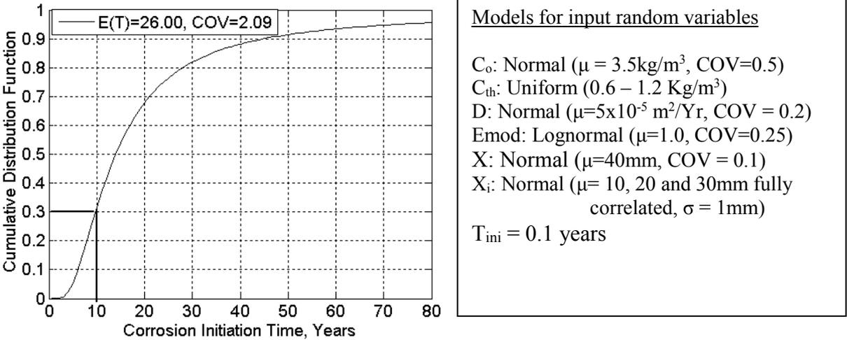
Figure 1: Distribution for the corrosion initiation time.
