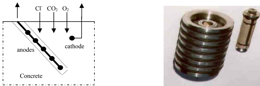
Figure 3: Sensors for corrosion risk monitoring a) Ladder arrangement b) Expansion Ring
