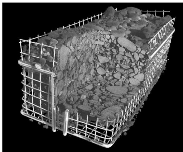
**Figure 1-** Example of a cut through 3D CT scan captured of a sediment core taken post flood event. Voxel resolution is 3mm and microplastic nurdles are identified in the scans from the differential density and hence the intensity of the return signal
