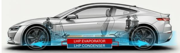
Figure 1. Idea of the proposed BTMS, where the condenser of the LHP is cooled by aerodynamic forced convection (image modified from ImageFX).
