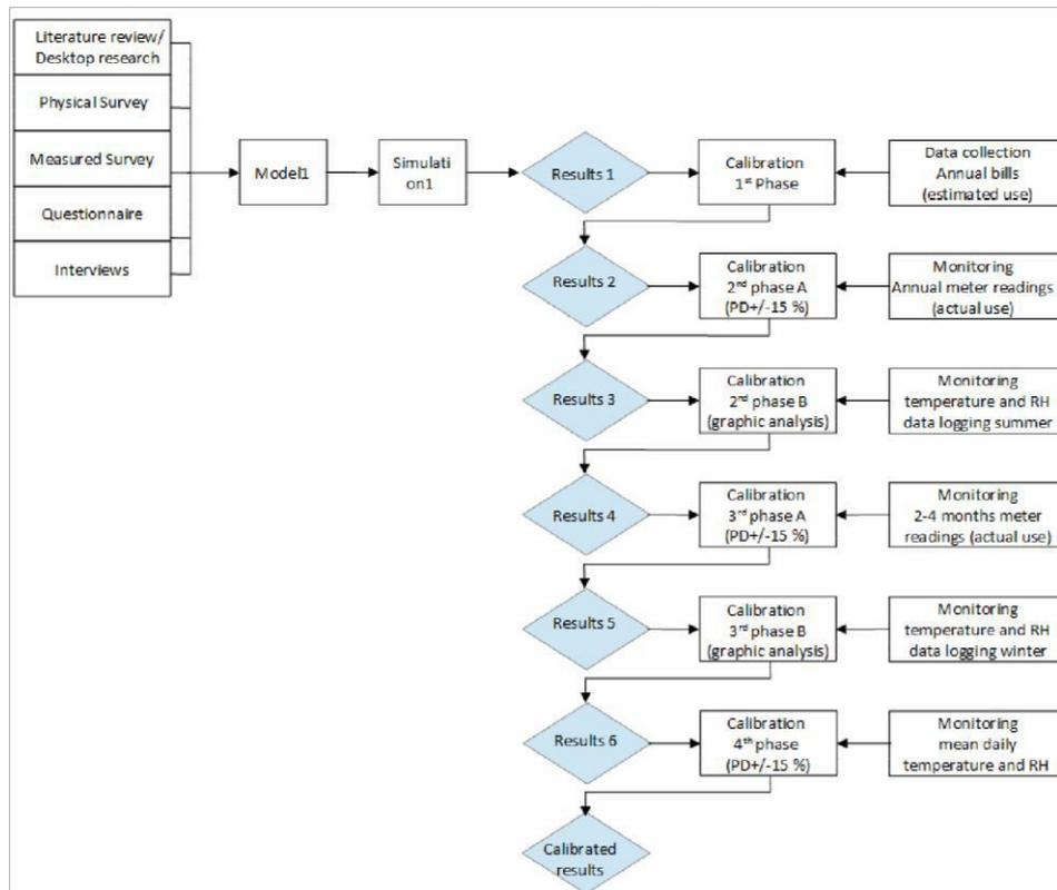
Figure 2. Flowchart of the calibrated simulation path as operated in the study.
