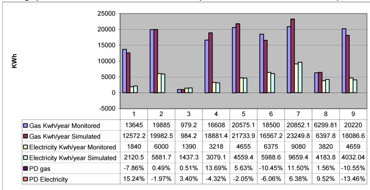
Figure 3. Graph and table showing the annual gas and electricity consumption (in Kwh) monitored and simulated for each CS (1-9) and the PDs calculated between them.
