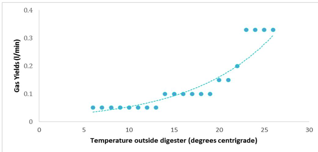
Figure 2. Gas yield variation of an anaerobic digester with temperature (based on [27]), including a trend line.
