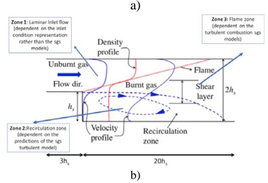
Figure 1: a) Experimental set-up of the backward facing step combustor [4] b) Schematic of the combustor simulation geometry and flow features
