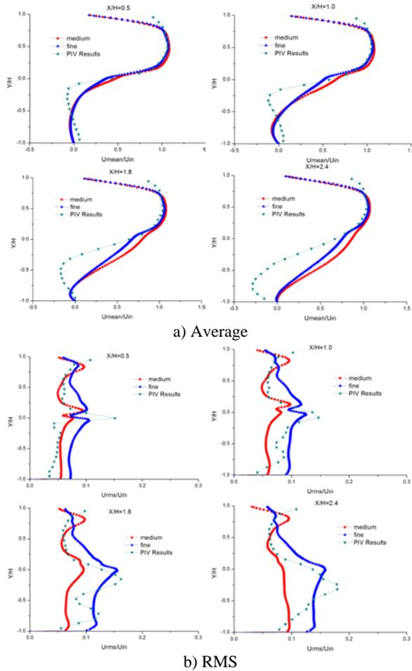
Figure 6 Axial velocity profiles for reacting cases
