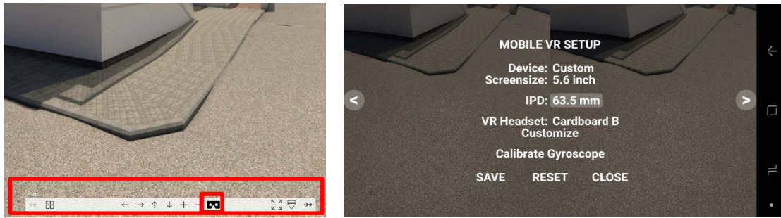
Figure 8: a) Enabling the stereoscopic view and, b) calibrating the mobile device and user viewing preferences for VR
