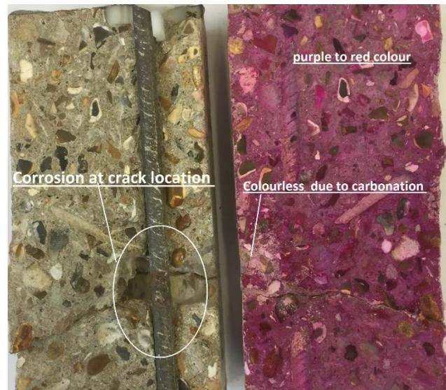
**Fig.10.** Corrosion of reinforcement bar at location of crack due to expose to CO<sub>2</sub> with 65% of RH
