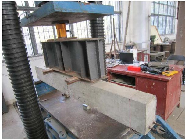
Figure 3. Flexural testing setup
