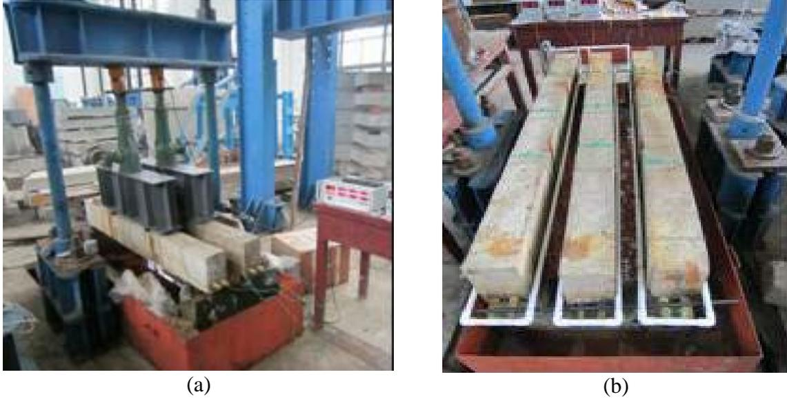
Figure 2. Test setup for (a) sustained loading, and (b) water spray for corrosion
