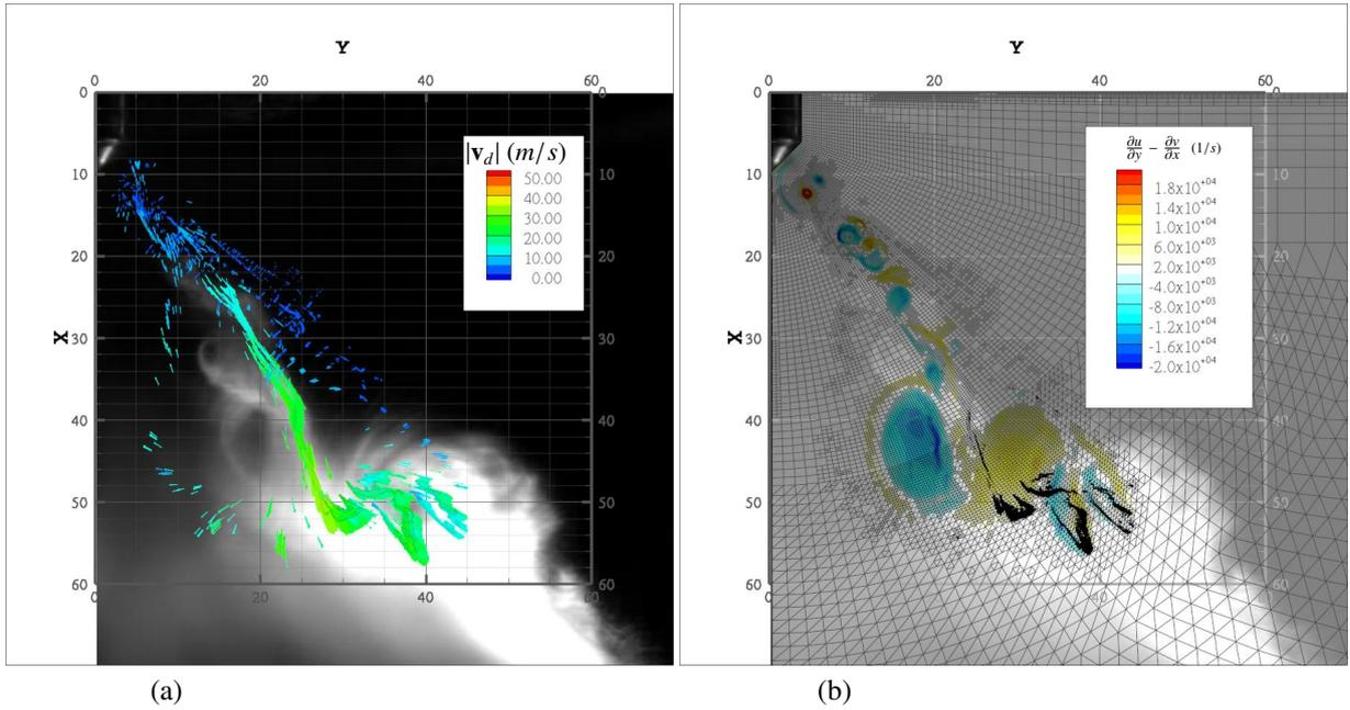
Figure 23: Comparison of the experimental observations of droplet distribution from [90] (shadow graphs) with the numerical results. (a): Droplet distribution at  $t = 1.67$  ms. Colour scale corresponds to velocity magnitude ( $m/s$ ). Scatter size corresponds to the number of droplets per parcel. (b): Distribution of the z-component of the vorticity vector in ( $1/s$ ) at  $t = 1.67$  ms.
