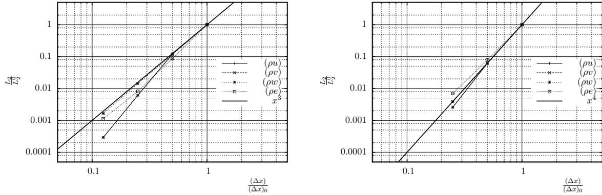
Figure 10: Values of the  $L_2$  error for the momentum components and energy, normalised by the value of the error for the coarse discretisation, versus mesh resolution for hexahedral elements. **Left:** Third order discretisation ( $p = 2$ ). **Right:** Fourth order accurate discretisation ( $p = 3$ ).
