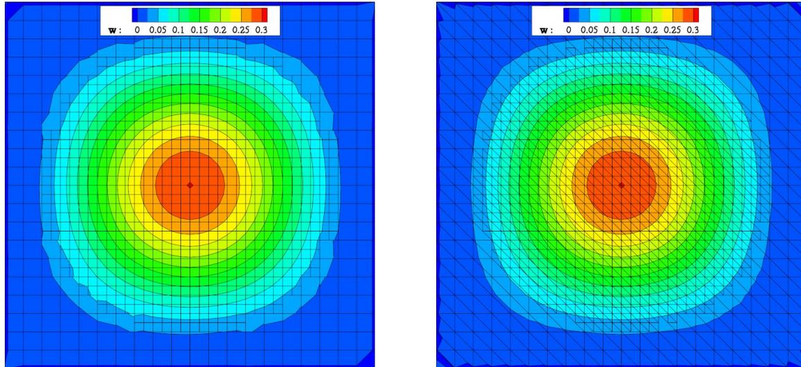
Figure 8: The final distribution of the  $w$  velocity for a square subdomain of the manufactured solution field with size  $L/2$  **Left:** For a spatially refined unstructured hexahedral mesh. **Right:** For a spatially refined unstructured prismatic mesh.
