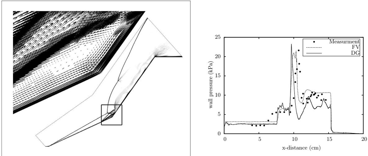
Figure 18: **Left:** Magnitude of the density gradient for the double cone simulation. **Right:** Pressure distribution along the wall of the double cone. Solid curve: reactive simulation. Dashed curve: reactive simulation by Nompelis [81] using the finite volume (FV) method. Dots: experimental data taken from [81].
