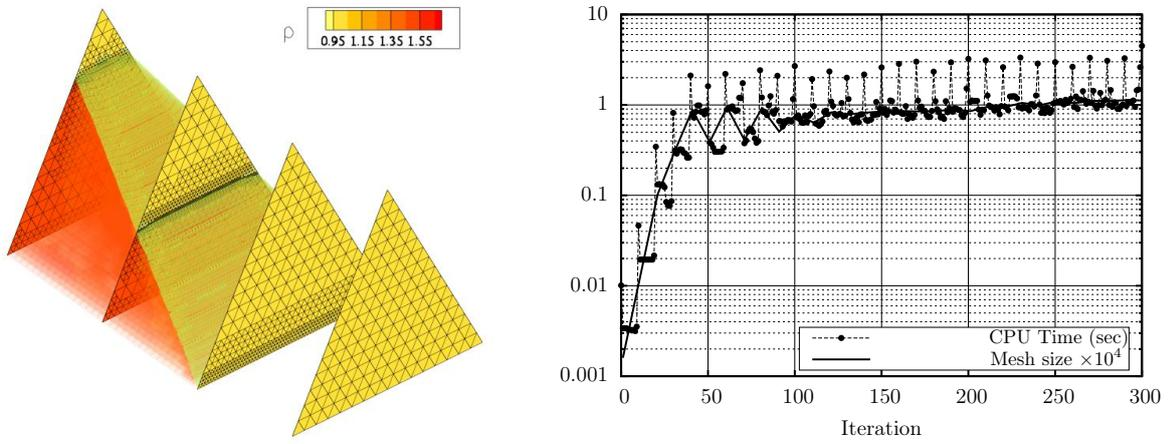
Figure 13: **Left:** Density distribution for the oblique shock problem discretised with prismatic elements. Light (yellow) iso-surface indicates the  $\rho = 1.05$  contour. **Right:** Performance of the AMR algorithm for the three dimensional oblique shock simulation using oct-trees. (Solid curve): CPU time for each timestep. (Dashed curve): Number of elements.
