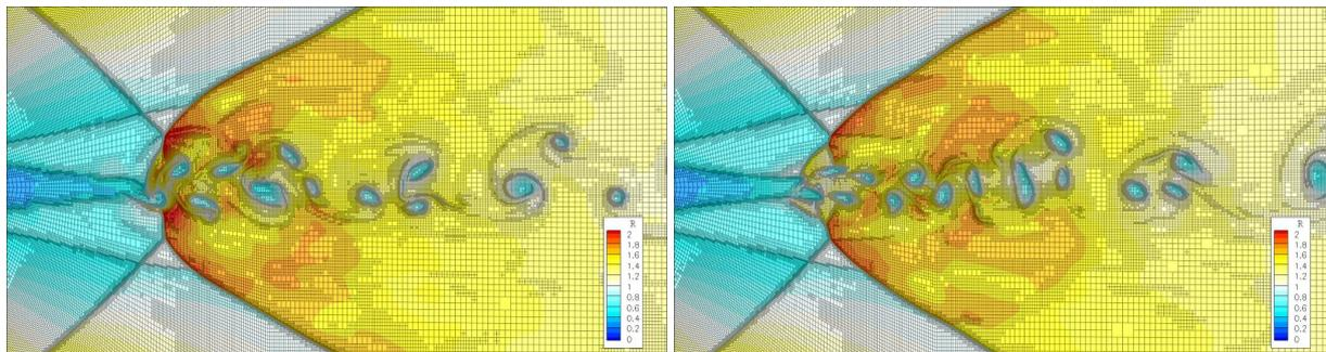
Figure 17: Density distribution at the wake of the cylinder where the reflected shocks interact for two time instants:  $t = t_1$  (**Left**) and  $t = t_1 + \Delta t$  (**Right**), for  $\Delta t = 1t^*$ .
