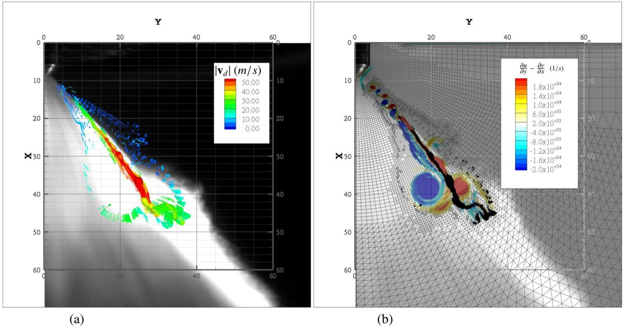
Figure 21: Comparison of the experimental observations of droplet distribution from [90] (shadow graphs) with the numerical results. (a): Droplet distribution at  $t = 1.1$  ms. Colour scale corresponds to velocity magnitude ( $m/s$ ). Scatter size corresponds to the number of droplets per parcel. (b): Distribution of the z-component of the vorticity vector in ( $1/s$ ) at  $t = 1.1$  ms.
