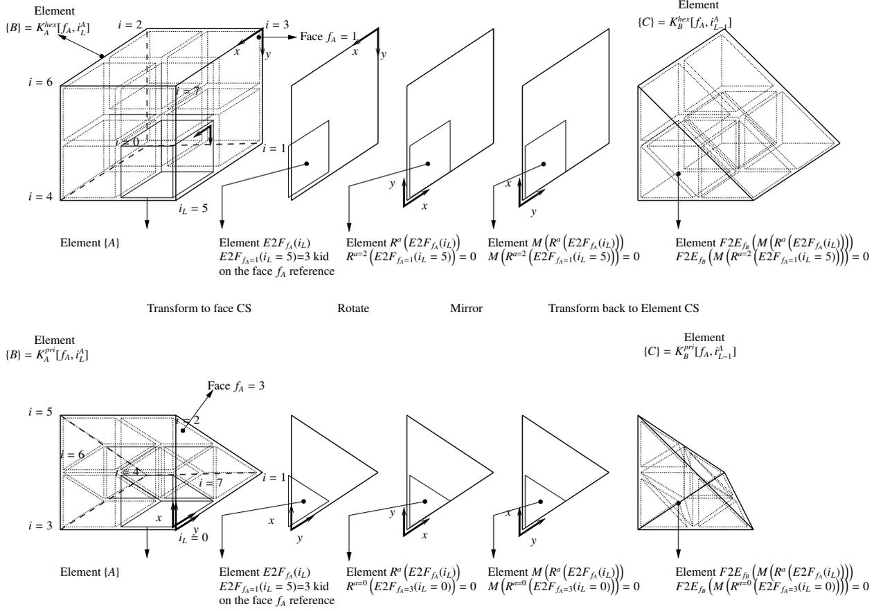
Figure 5: **Top:** Identifying the neighbouring element of a split element at a hexahedral to prism of oct-tree splitting, incorporating a rectangular face. **Bottom:** Identifying the neighbouring element of a split element at a prism to tetrahedron of oct-tree splitting, incorporating a triangular face.
