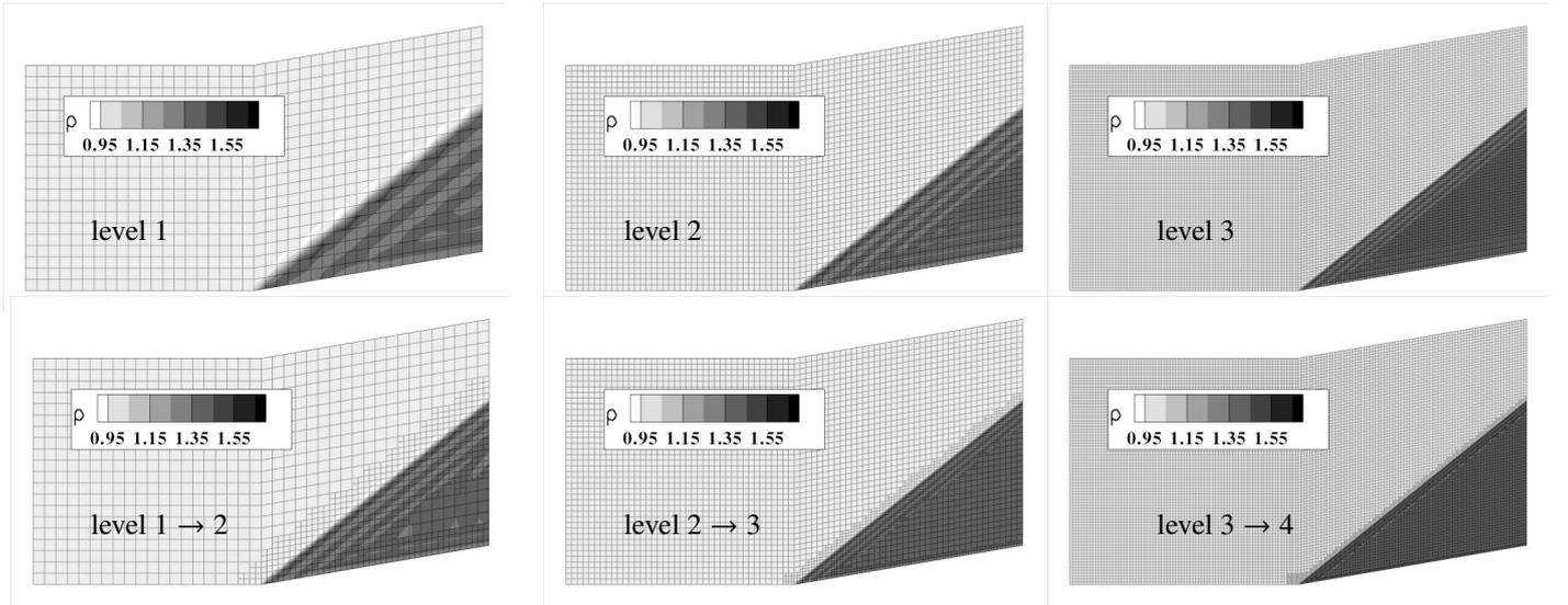
Figure 11: Density distribution for the converged numerical solutions to the oblique shock problem. **Top:** Level 1, Level 2 and Level 3 solutions on a uniform hexahedral mesh. **Bottom:** Converged AMR solutions restarted from the corresponding solutions in the upper row.
