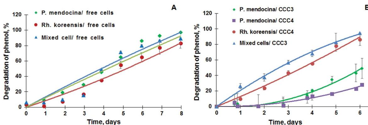
Fig. 6 (A) Degradation of phenol by the suspension of *P. mendocina*, *Rh. koreensis* and their mixture (1 : 1). ( $n = 2$ ), (B) degradation of phenol by *P. mendocina* CCC3 and CCC4 with a crosslinked number of cells equal to  $5 \times 10^9$ , *Rh. koreensis* CCC4 and their mixture CCC3 (1 : 1) ( $n = 2$ ).
