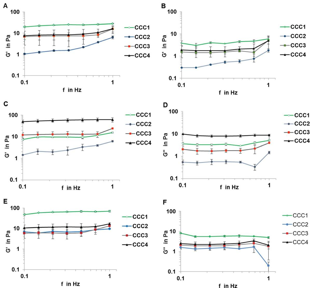
Fig. 5 Rheology diagrams for all bacterial strains *P. mendocina* (A and B), *Rh. koreensis* (C and D) and mixed cultures (E and F) crosslinked with four cross-linked polymer solutions CCC1, CCC2, CCC3 and CCC4. ( $n = 3$ ).
