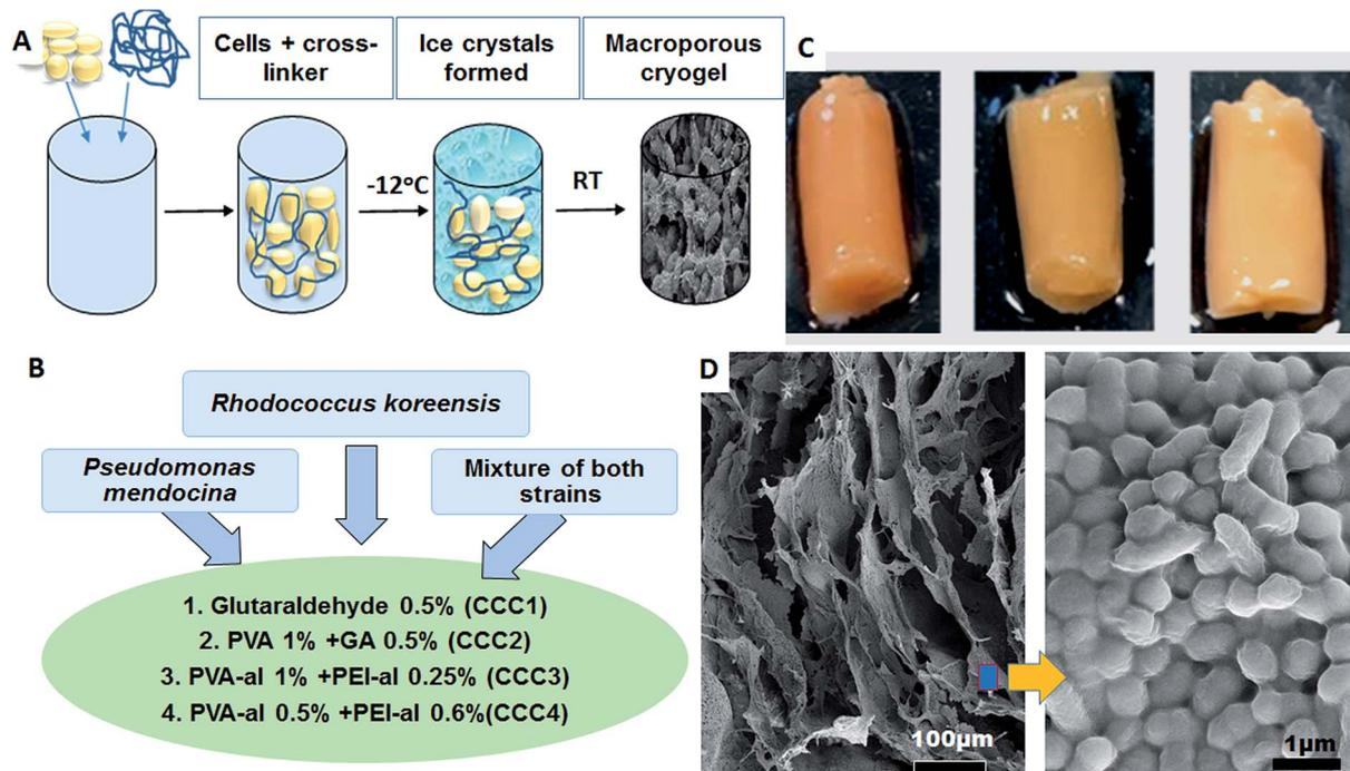
Fig. 2 (A) Scheme of cryogel preparation, (B) types of bacterial strains and four cross linker polymer solutions used, (C) CCC4 of *P. mendocina* (left), *Rh. koreensis* (middle) and mixed cells (right), (D) SEM images of *P. mendocina* cross-linked in CCC4.
