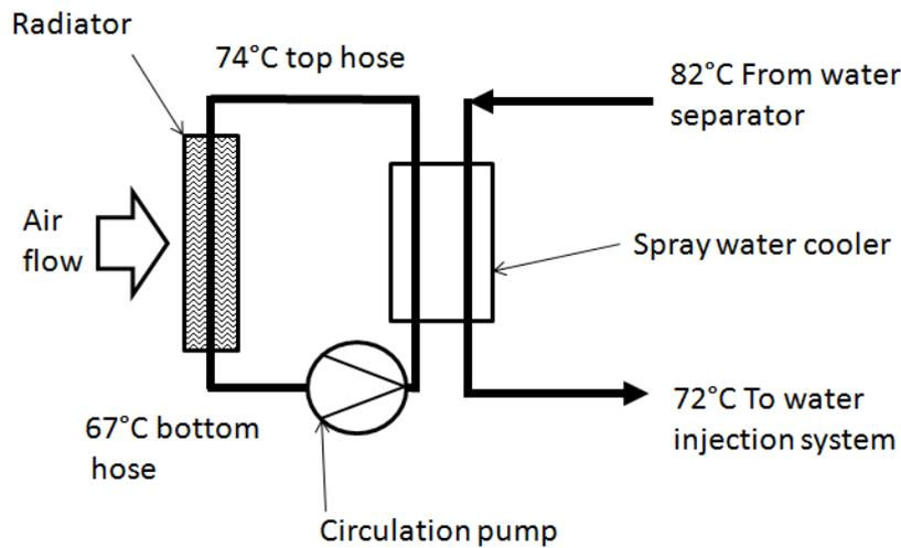
**Figure 5: Spray water cooling circuit**
