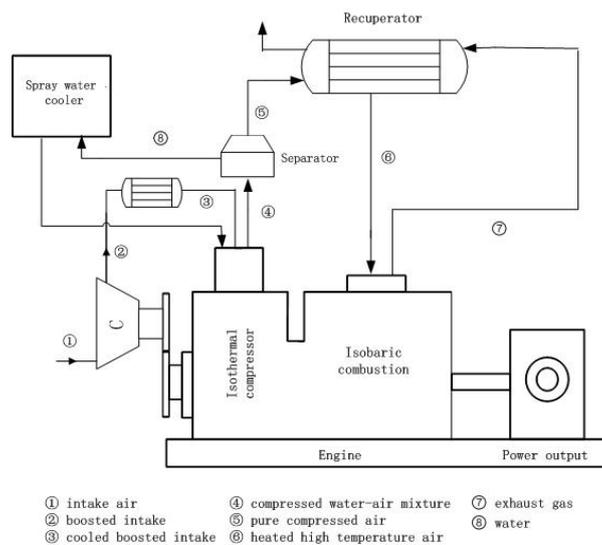
**Figure 1: Schematic of a split cycle engine**
