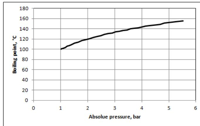
**Figure 4: Relationship between boiling point and pressure for water**
