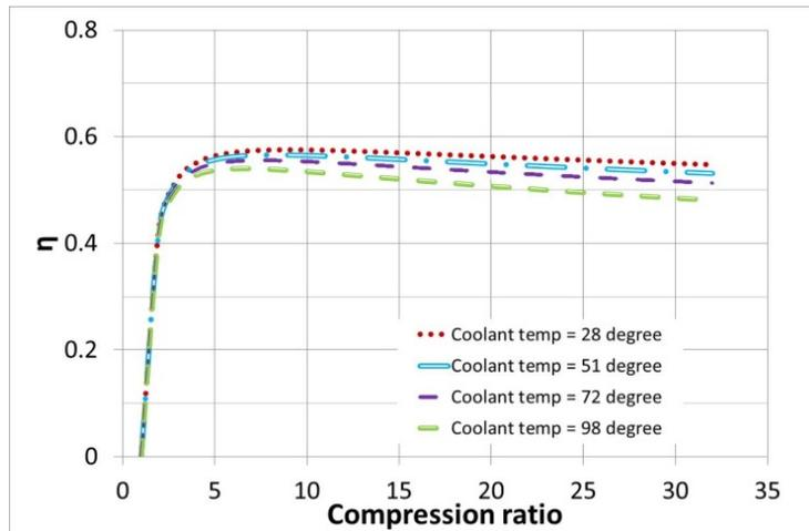
**Figure 2. Effect of spray water temperature on cycle efficiency as a function of compression ratio**
