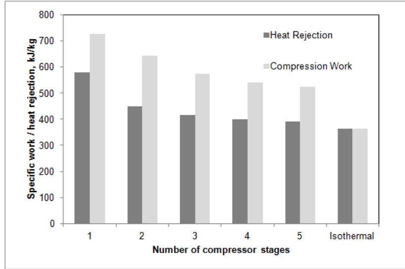
**Figure 3: Comparison of work and heat rejection from multi stage compression to achieve 110 bar pressure**
