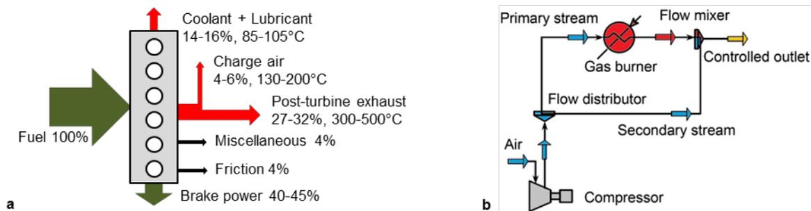
**Figure 1: (a) Fuel energy distribution in the mid to large scale engines at relatively higher speeds and loads, (b) Schematic of the experimental heat source setup**
