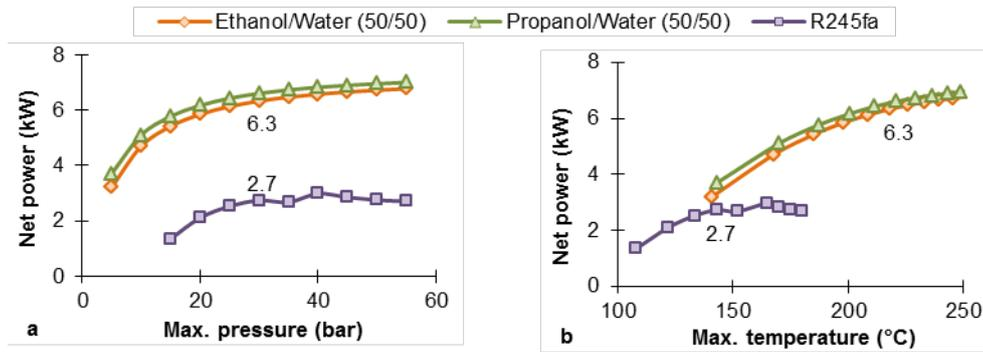
**Figure 3: Comparison of theoretical net power between R245fa and alcohol-water blends at (a) Maximum cycle pressure, and the corresponding (b) Maximum cycle temperature**
