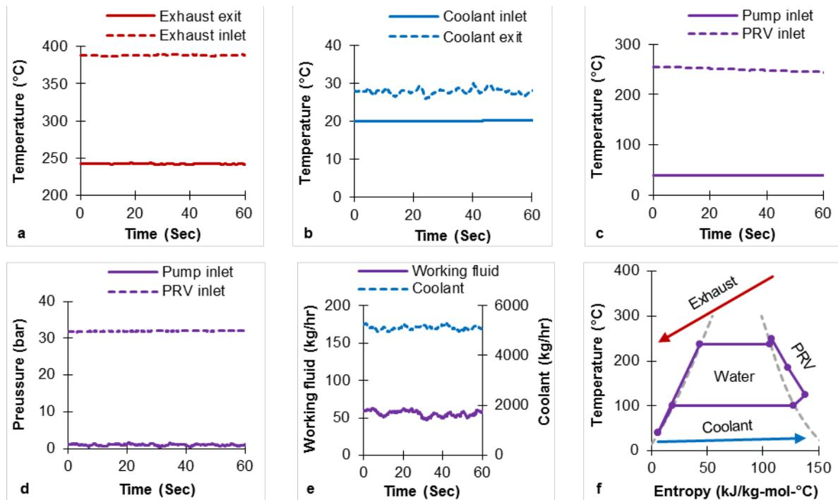
**Figure 6: Off-design steady-state test results (a) Source quality, (b) Sink quality, (c) Working fluid temperature limits, (d) Working fluid pressure limits, (e) Working fluid and coolant flow rates, (f) T-S diagram of the process using a PRV**
