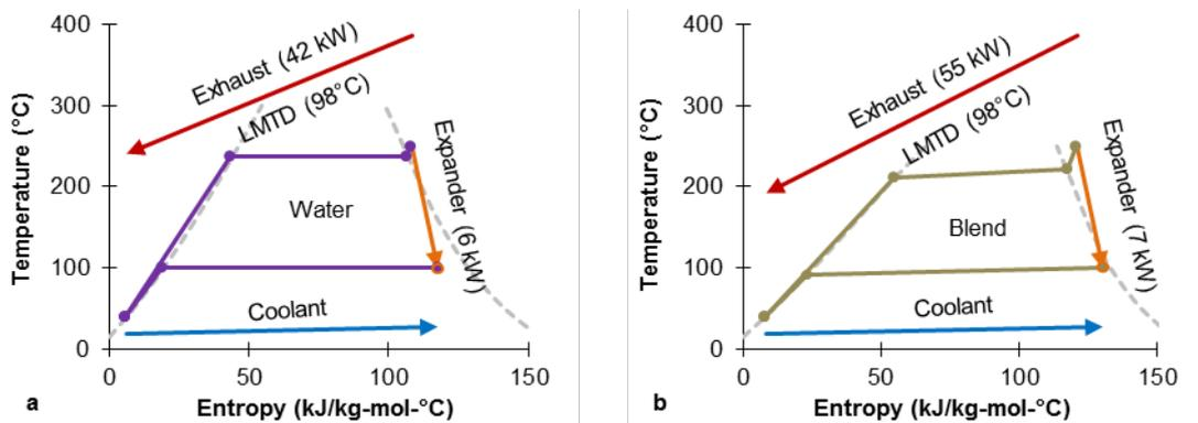
**Figure 7: (a) Potential T-S diagram when integrating a high-pressure ratio expansion process
