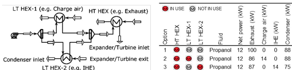
**Figure 4: Schematic of the experimental heat recovery architecture and normalised comparison of the architecture options**
