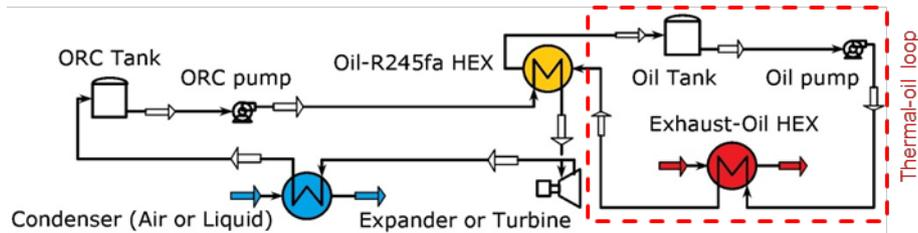
**Figure 2: Schematic of a thermal-oil loop coupled with a conventional ORC**
