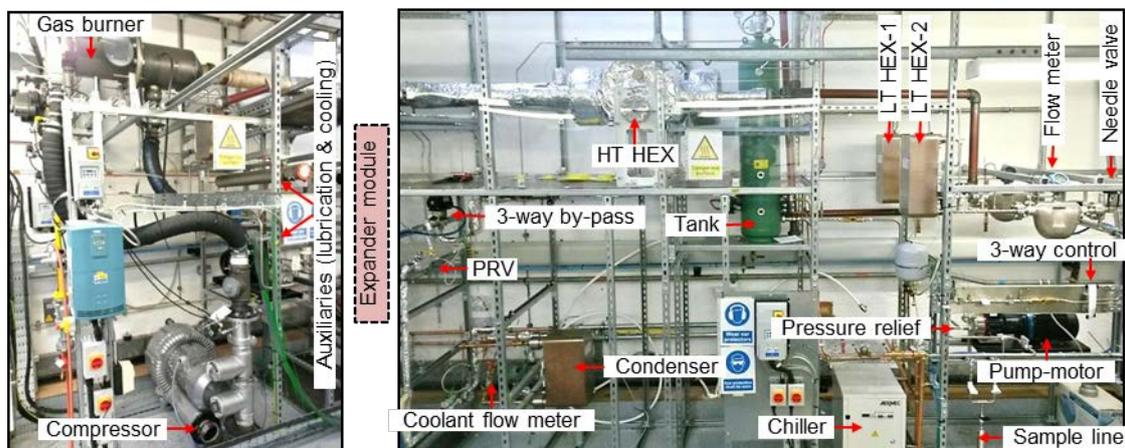
**Figure 5: High-temperature high-pressure ORC facility employing three heat exchangers in mixed series and parallel combination for alcohols and alcohol-water blends**
