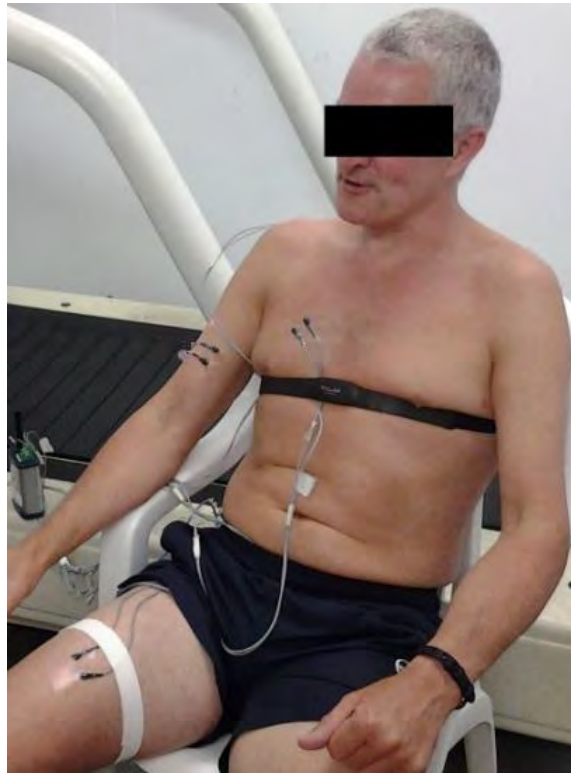
Figure 26: showing location of thermistors on chest, upper arm and thigh. Thermal camera measurements were taken beside the thermistors, ensuring the patches did not interfere with measurement.
