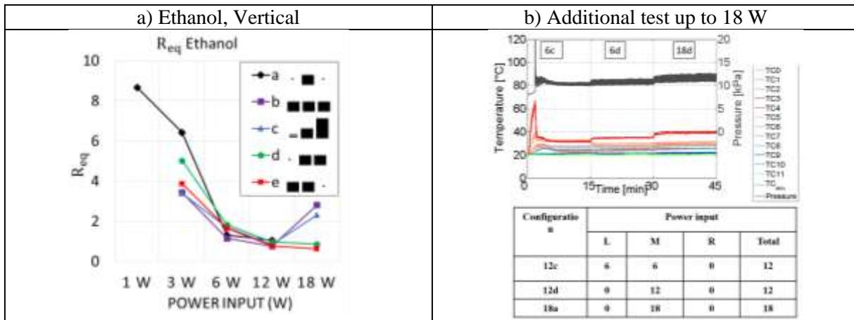
Figure 4. a) Equivalent Thermal Resistance for all the heating distribution tested for long test with Ehanol in vertical position and b) Test performed providing to the device up to 18 W solely at the heater M.
