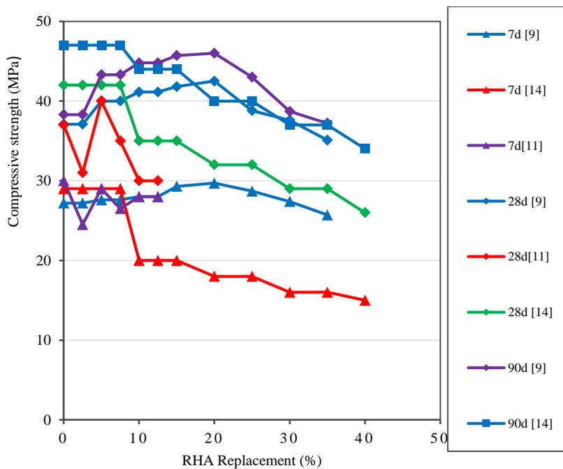
Fig. 3. Compressive strength of RHA blended concrete from [9] [10] [13] [14].
