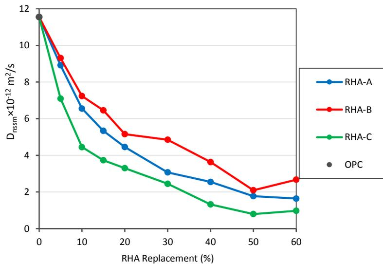
Fig. 5. Chloride ion diffusion of RHA concrete after 28 days.
