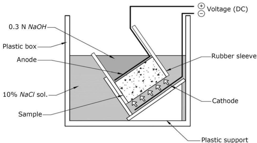
*Fig. 1. The non-steady state migration test set-up: Anolyte (0.3M NaOH), Catholyte (10% NaCl) [1].*
