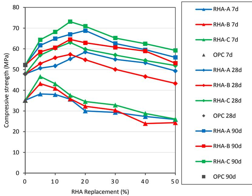
Fig. 2. Compressive strength of control and RHA blended concrete.
