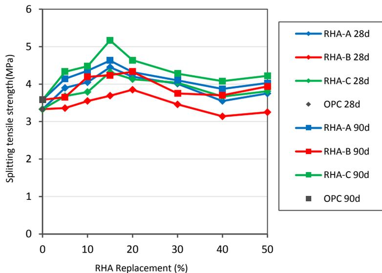
Fig. 4. Splitting tensile strength of control and RHA blended concrete.
