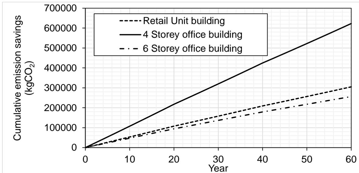
Figure 5. Reduction in CO<sub>2</sub> emissions for three buildings studied
