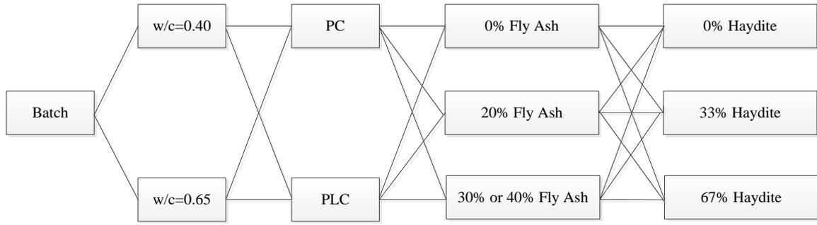
Fig.1 Experimental design of 36 concrete batches
