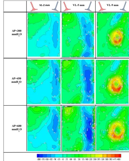
Fig. 4. Vorticity Magnitudes at Different valve lifts and Pressure Differences.
