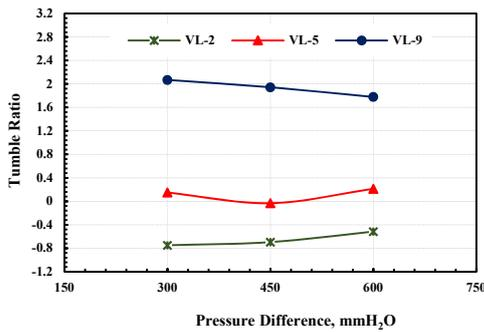
Fig. 5. Evolution of the tumble ratio as a function of the pressure difference and the valve lift.
