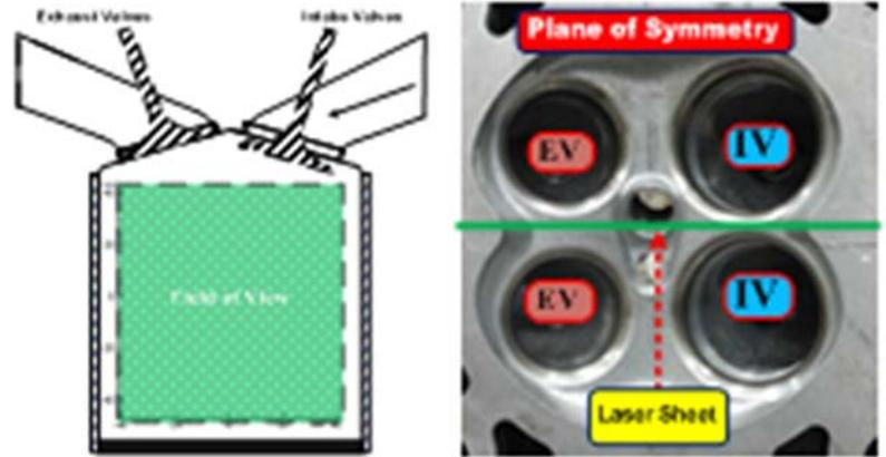
Fig. 2. Mid-cylinder plane (plane of symmetry)
