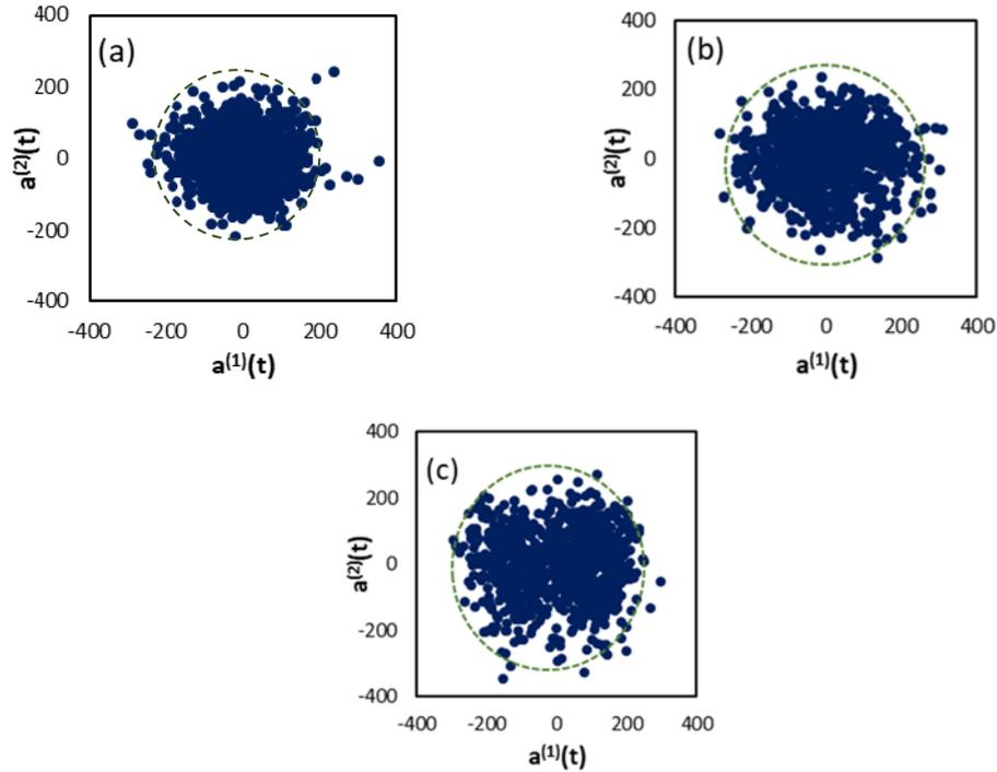
**Fig. 9.** POD coefficients for modes 1 and 2 at valve lift 9 (a)  $\Delta P=300$  mmH<sub>2</sub>O, (b)  $\Delta P=450$  mmH<sub>2</sub>O, (c)  $\Delta P=600$  mmH<sub>2</sub>O.
