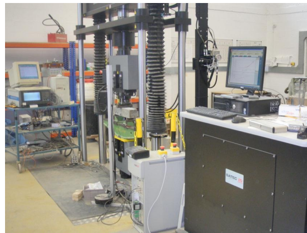
Figure 2. Servo-hydraulic Closed-loop Testing Machine
