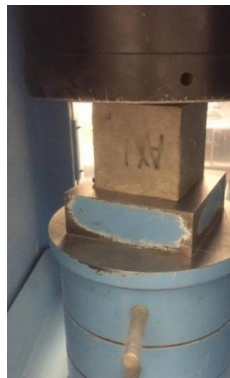
Figure 2. Compressive strength test
