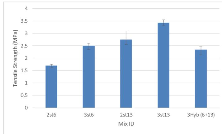
**Fig. 5.** Tensile strength of steel fibre reinforced geopolymer composite (SFRGC)
