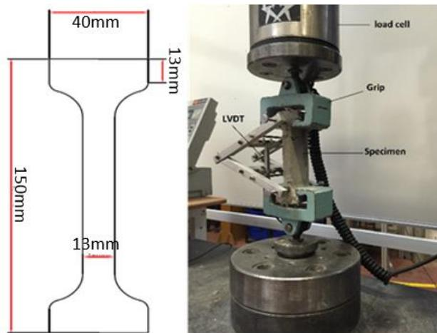
**Fig. 2.** Experimental set up for (left) dog bone specimens and (right) tensile strength test set up
