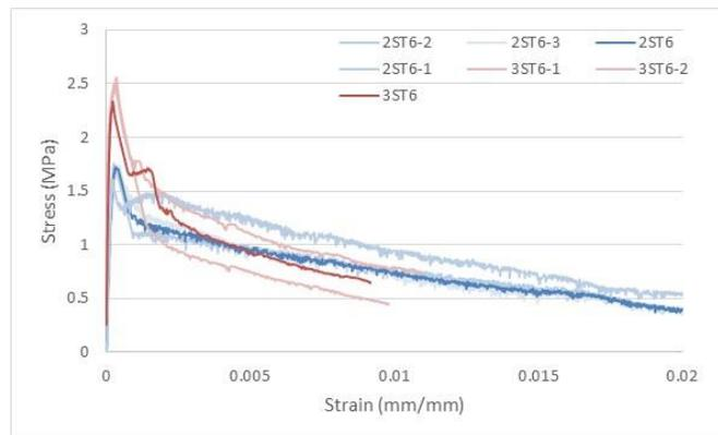
**Fig 4a.** Tensile stress-strain response of SFRGC -6mm with 2%  $V_f$  and 3%  $V_f$ .
