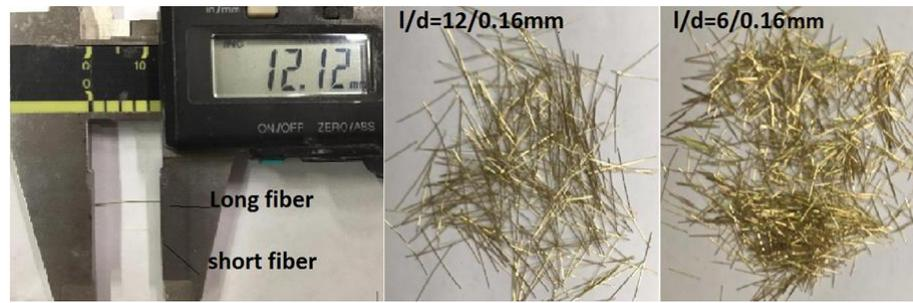
**Fig. 1.** Steel fibres used in this study
