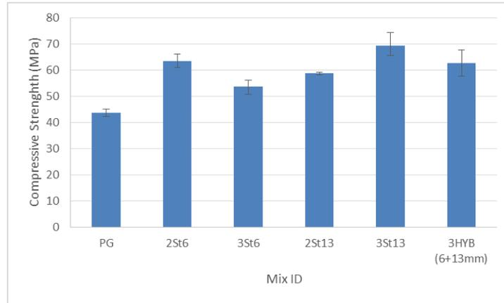
**Fig. 3.** Compressive strength of steel fibre reinforced geopolymer composite (SFRGC)
