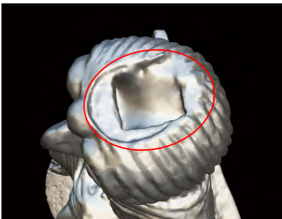
Figure 2: Head of ‘Horus’ 3dDM showing a square hole whose geometry was only partially captured.
