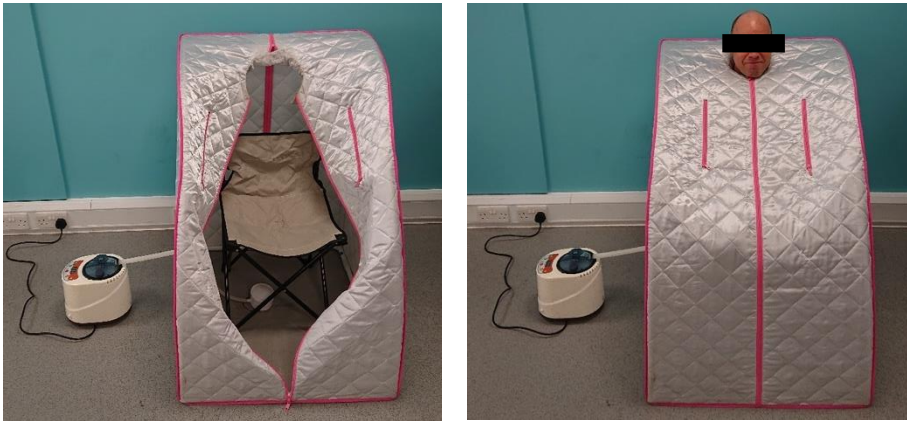
588 Figure 1. The portable steam sauna pod system (left: image of open portable sauna with seat inside and 589 water steam container outside, right: image with participant inside the sealed system).
