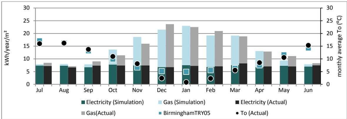
Fig 7. Monthly measured and simulated energy consumption
