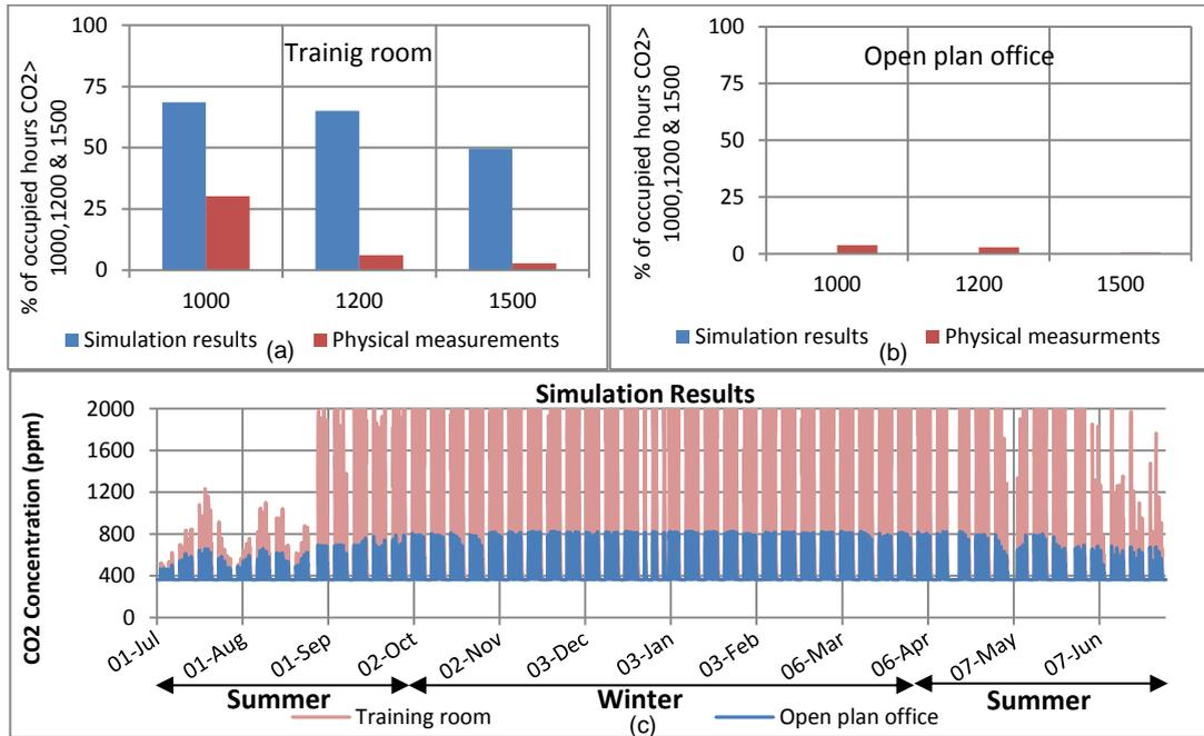
Fig 5. CO<sub>2</sub> concentration in measured and simulated models
