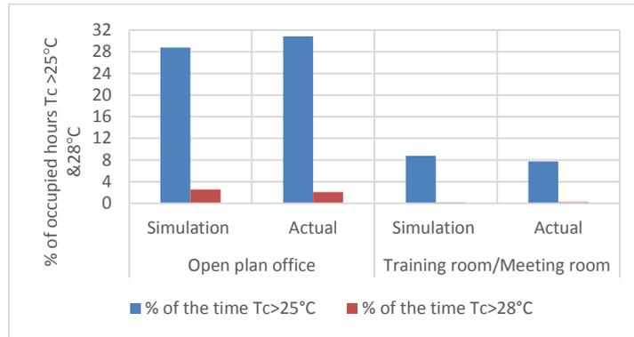
Fig 3. Frequency of the time when operative temperature is higher than 25°/28 °C in both actual building and computer model for the base case
