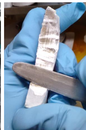
Fig. 5. Sodium with external layer partially removed.
