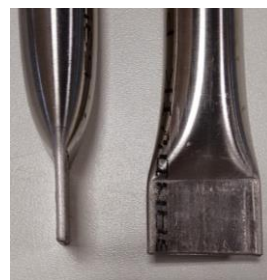
Fig. 2. Smashed tube end.
