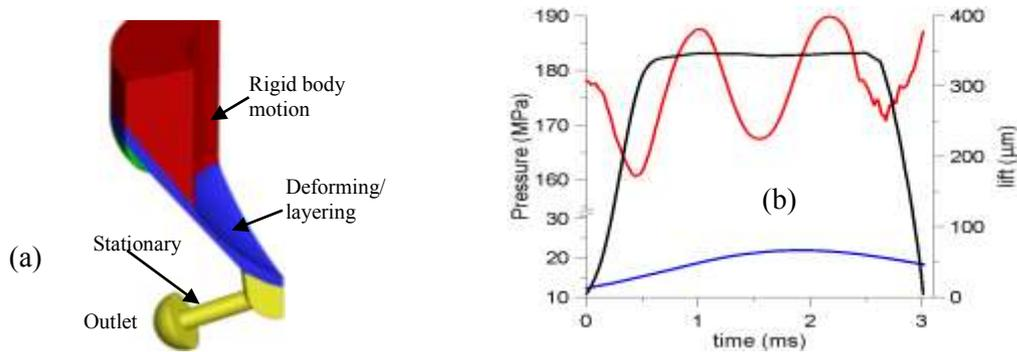
Fig. 1. (a) Grid partitioning of the 1/5<sup>th</sup> sector of the injector examined, (b) needle lift, injection and back pressure profiles considered in the simulations
