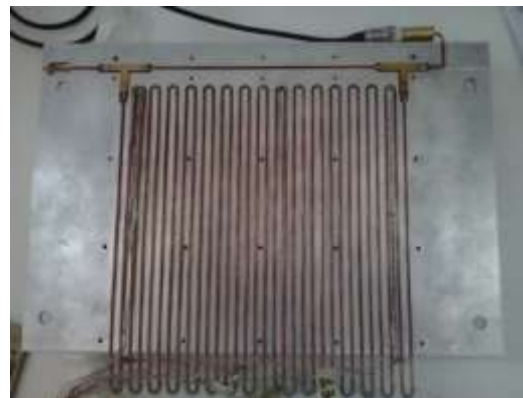
Figure 2: heat sink embedded PHP with pressure sensor and thermocouples.
