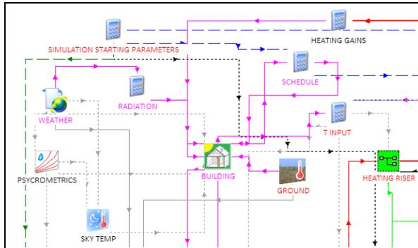
Figure 1 Extracted view of the Trnsys HVAC model
