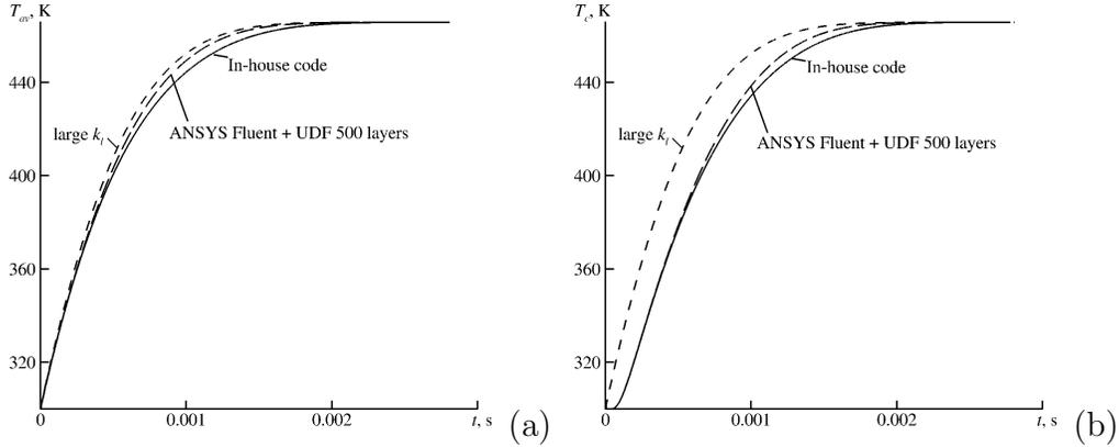
Figure 3: *n*-Dodecane droplet heating and evaporation. Initial droplet temperature is 300 K, temperature of air is 650 K: (a) evolution of the droplet average temperature; (b) evolution of the temperature in the centre of the droplet. Solid curves – in-house code, long dashed curves – case 1, dashed curves – case 3.
