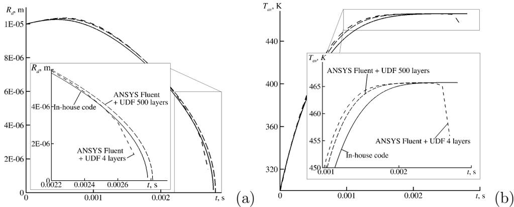
Figure 1:  $n$ -Dodecane droplet heating and evaporation. Initial droplet temperature is 300 K, temperature of air is 650 K: (a) evolution of the droplet radius; (b) evolution of the droplet average temperature. Solid curves – in-house code, long dashed curves – case 1, dashed curves – case 2.
