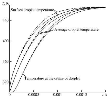
Figure 2: *n*-Dodecane droplet heating and evaporation. Initial droplet temperature is 300 K, temperature of air is 650 K: evolutions of the temperatures in the centre of the droplet, at the droplet surface, and of the average temperature. Solid curves – in-house code, long dashed curves – case 1.
