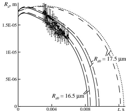
Figure 4: *n*-Dodecane droplet heating and evaporation. Experimental data vs ANSYS Fluent predictions. Triangles – experimental data: filled symbols – droplet 1, hollow symbols – droplet 2. Solid curves show theoretical predictions for  $T_{d0} = 380$  K,  $v_0 = 3.5$  m/s; long dashed curves –  $T_{d0} = 360$  K,  $v_0 = 3.5$  m/s; dashed curves –  $T_{d0} = 380$  K,  $v_0 = 0$  m/s; dotted curves –  $T_{d0} = 360$  K,  $v_0 = 0$  m/s.
