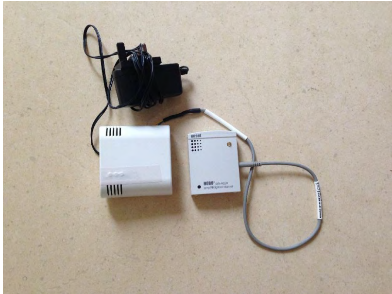
Figure 2: Hobo U12 data logger and CO 2 sensor
