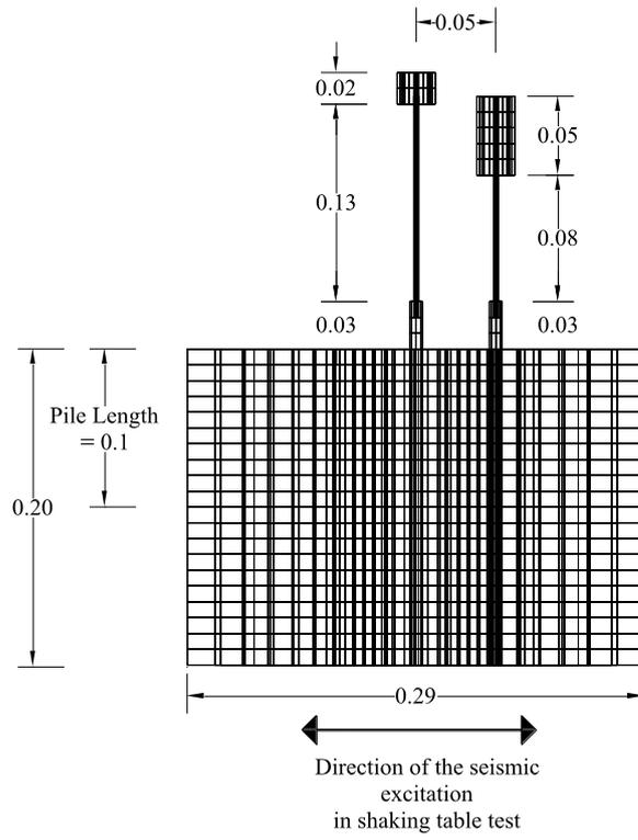
Figure 10 Set up of the experiment for shaking table (case with structure protected by ViBa device)
