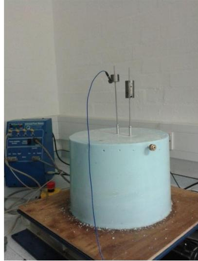
Figure 9 Test models realized in the laboratory and placed over a shaking table for a) single structure and b) structure coupled with ViBa.
